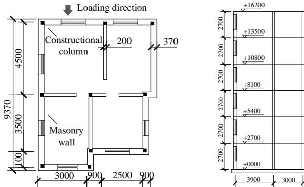
Fig. 7 – Layout of the RM structure (unit: mm)
