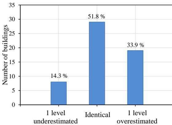
Fig. 11 – The comparison between the predicted damage states and actual damage states
