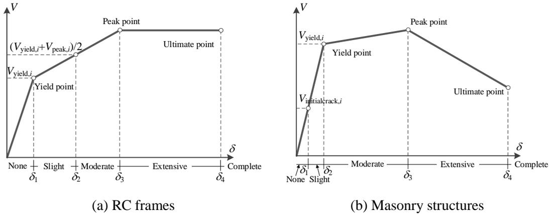
Fig. 4 – Inter-story backbone curves and damage limits
