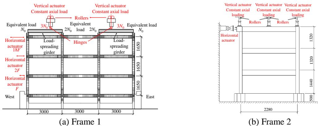
Fig. 5 – Test setup of the RC frames (unit: mm)
