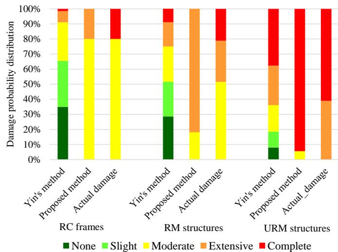
Fig. 12 – Comparison of predicted seismic damage and actual damage
