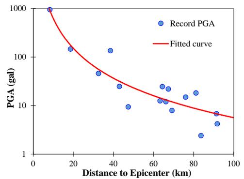
Fig. 10 – The attenuation function of Ludian earthquake
