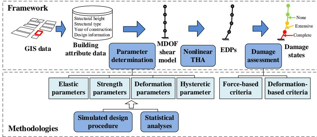
Fig. 1 – The framework and methodologies of the THA-based regional seismic damage prediction
