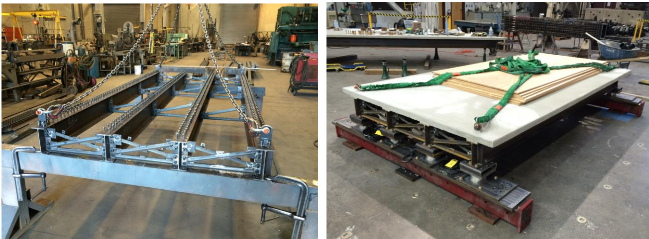
Fig. 2 – Steel bridge after the assembly of steel components at Reno Iron works (left) and composite bridge sitting on the bent caps in the Large Scale Structures Lab at the University of Nevada, Reno (right)
