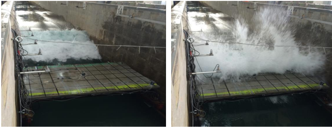
Fig.5 – Bore slightly before (right) and slightly after (left) impacting the bridge specimen
