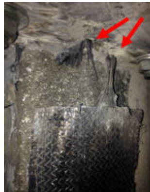
Fig. 9b. Mode of failure of specimen SW600C/1 No 1. Fracture of the CFRP rope.
