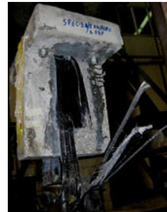
Fig. 9c. Mode of failure of specimen SW600C/1 No 1. Fracture of the CFRP rope.
