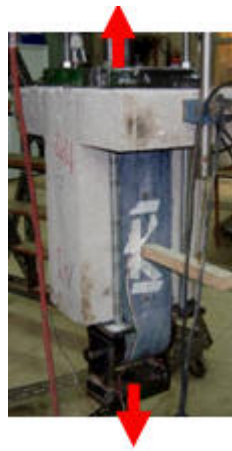
Fig. 4b. R/C units T-Beam with a CFRP strip being axially loaded.
