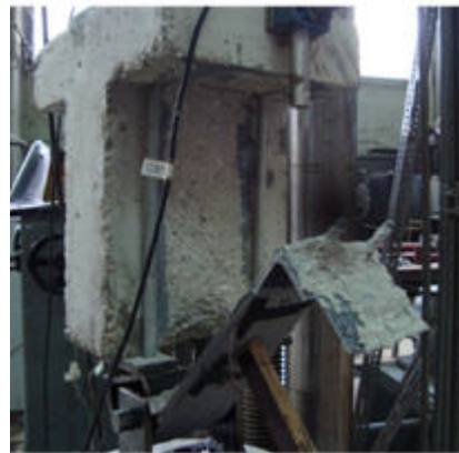
Fig. 6b. Failure of the anchoring scheme accompanied with debonding
