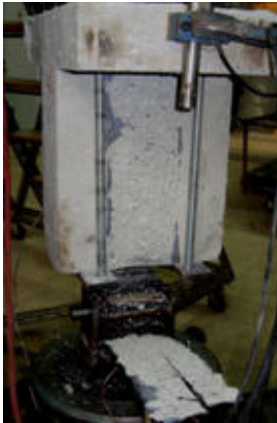
Fig. 6a. Debonding mode of failure
