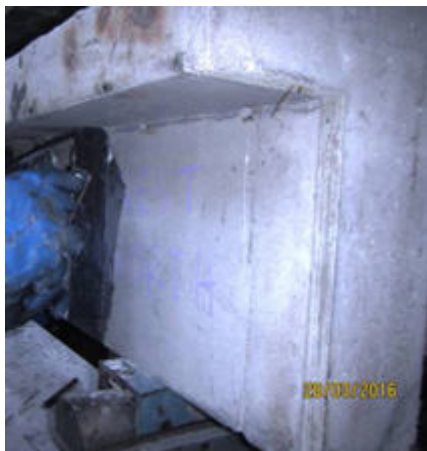
Fig. 4a. Prototype R/C T-Beam tested with or without external CFRP strips as shear reinforcement.
