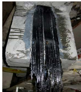
Fig. 10b. Failure mode of specimen CFRP strip Ref-1
