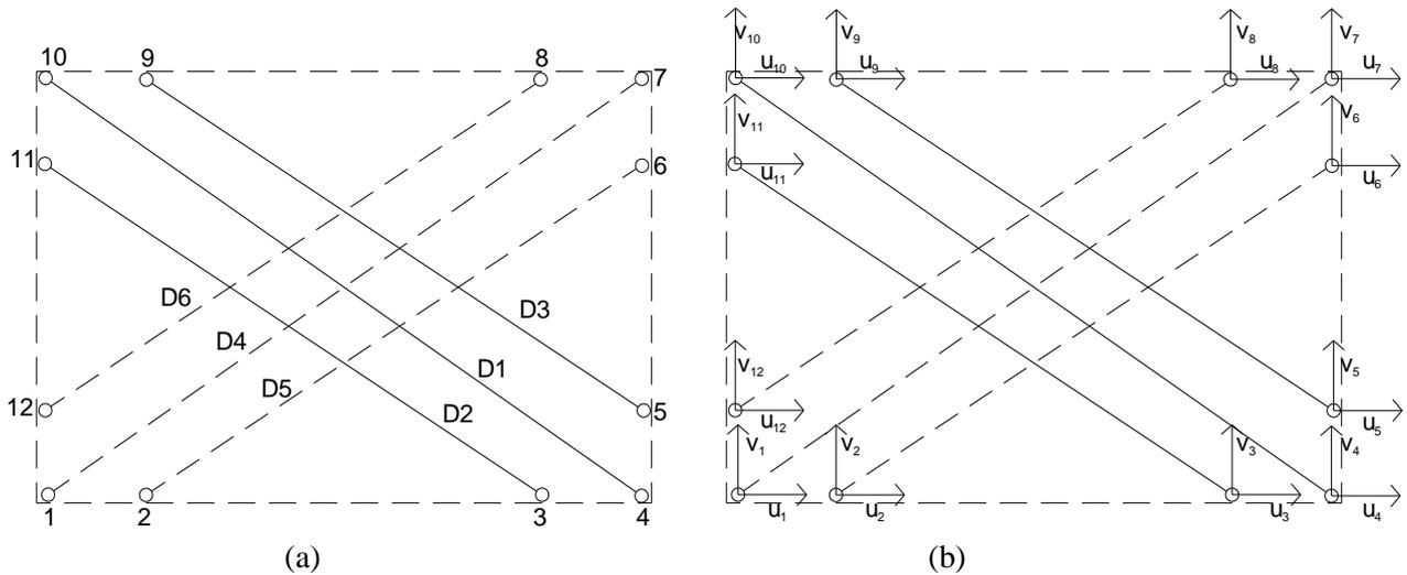
Fig. 1 – Macro-element for masonry panel: (a) nodes and struts, (b) degrees of freedom
