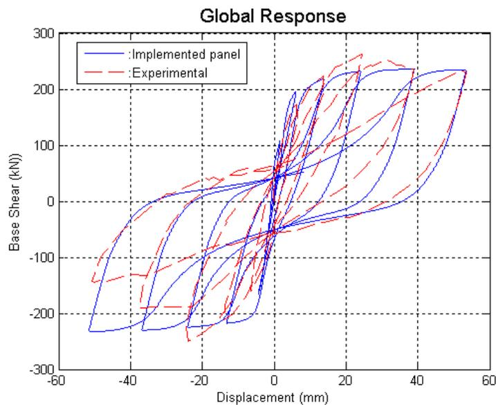
Fig. 12 – Comparison of experimental and analytical results from Wall U3 [17].
