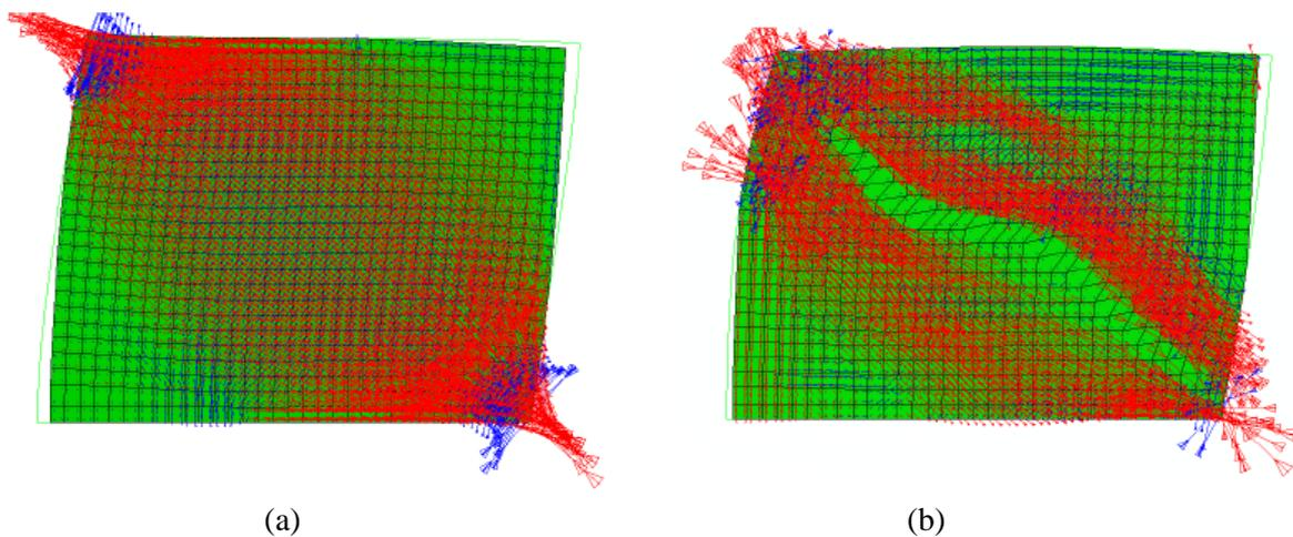
Fig. 4 – Principal stresses at (a) maximum shear and (b) post maximum point. [8]
