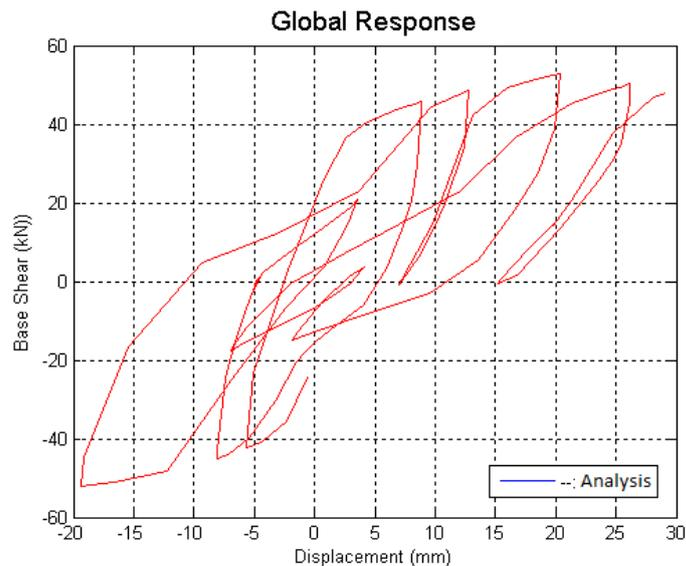
Fig. 14 – Dynamic response of 3D model.
