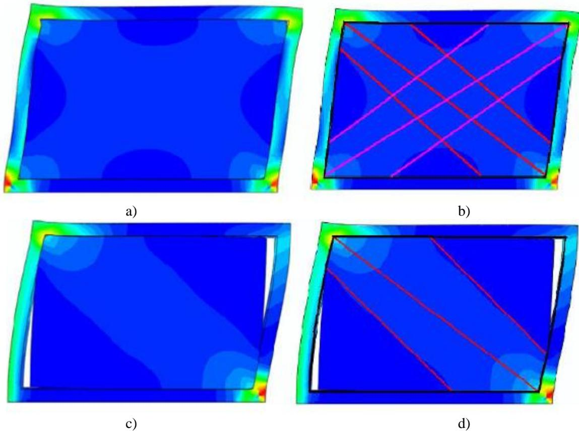
Fig. 3 – Deformed shape and Von Mises stresses in a finite element model of a confined masonry wall (a) at the initial stage, and (b) Initial stage with justification for three struts, (c) after separation, (d) after separation with struts [8]
