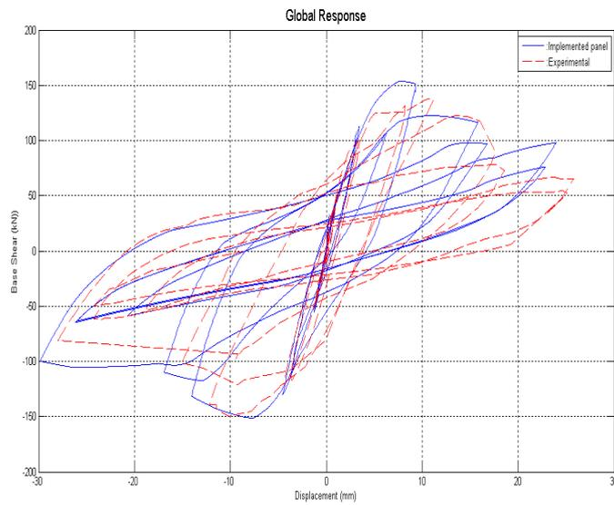
Fig. 6 – Comparison of experimental and analytical results from Wall M01 [13].
