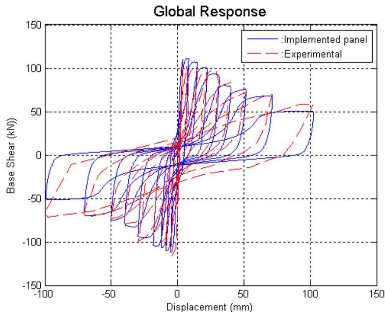
Fig. 8 – Comparison of experimental and analytical results from Wall M2 [16].
