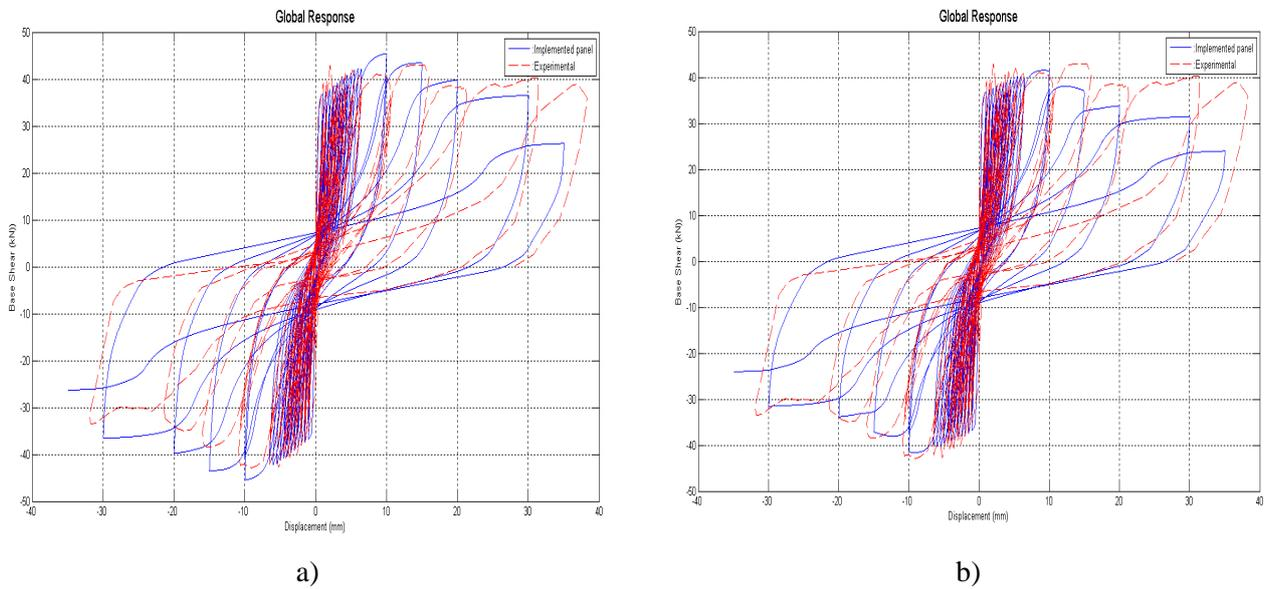
Fig. 10 – Comparison of experimental and analytical results from Specimen 1 [7].
