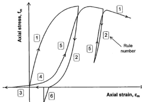
Fig. 2 – Hysteretic model used by the struts
