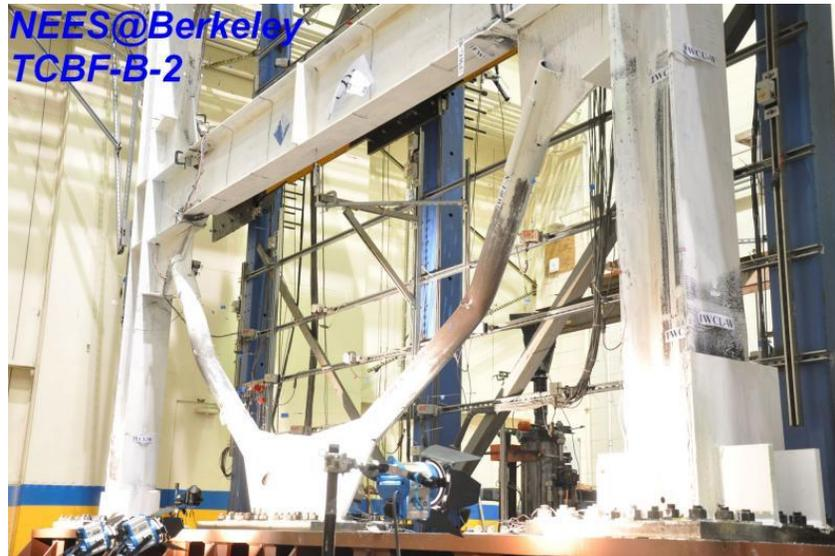
Fig. 6 –Experimental substructure in composed by braced frame system (NEES project 605, <https://nees.org/warehouse/project/605>)
