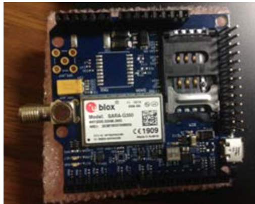
Fig. 6 – Coordinator with a GPRS protocol
