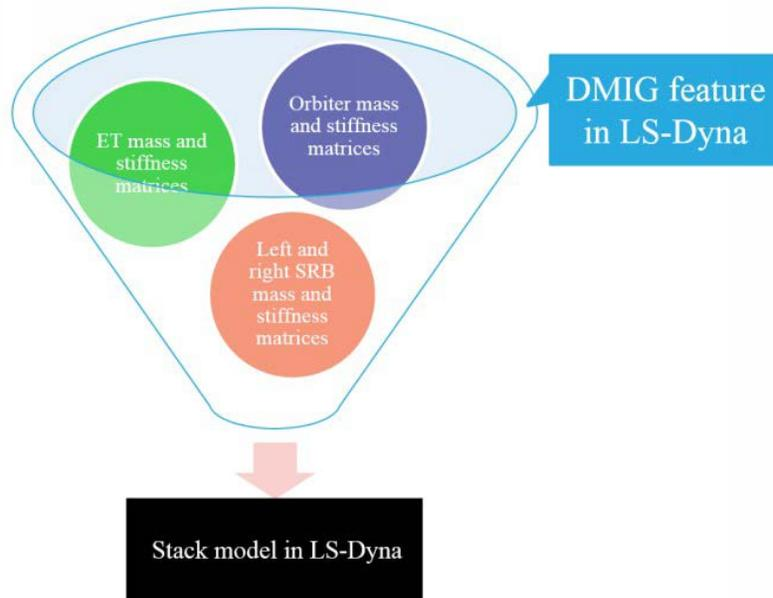
Figure 4 – Modeling the Stack in LS-Dyna
