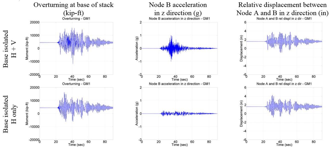
Figure 11 – Comparison between with and without vertical ground motion component
