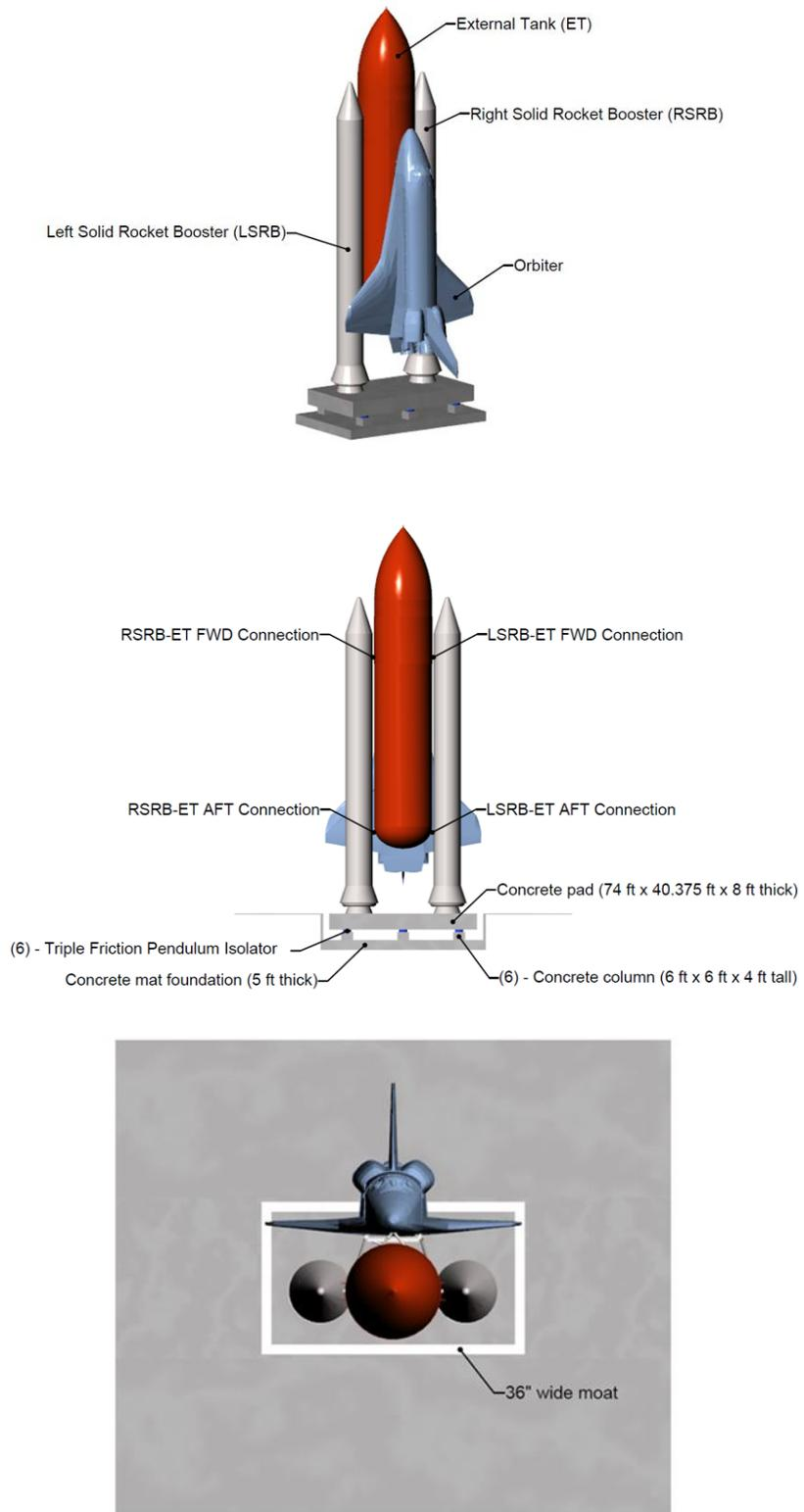
Figure 2 – Enlarged elevation view of the support structure by Arup
