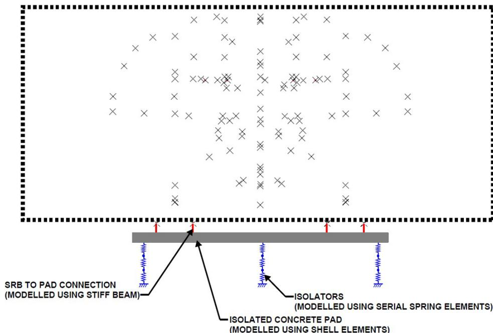
Figure 5 – Enlarged elevation view of the support structure
