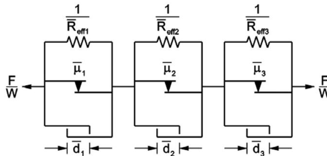
Figure 7 - Three single concave FP elements in series used to model the behaviour of the triple FP bearing
