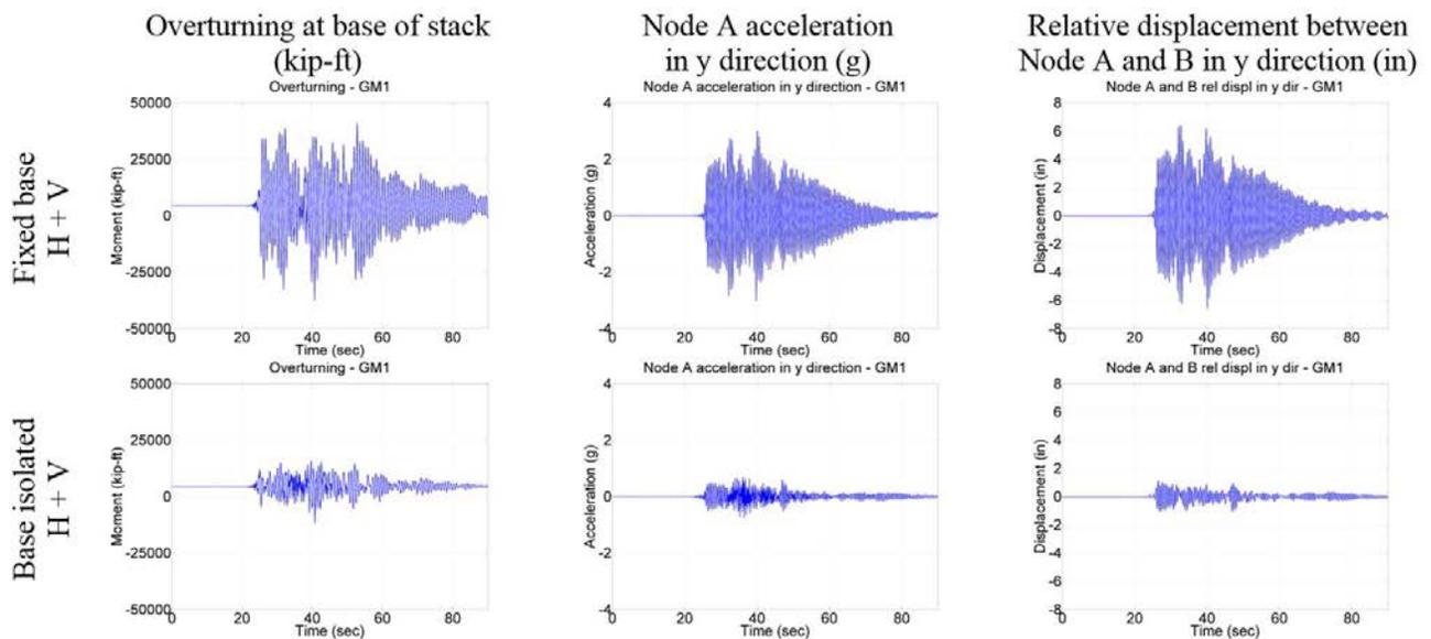
Figure 10 – Comparison between fixed base and base isolated
