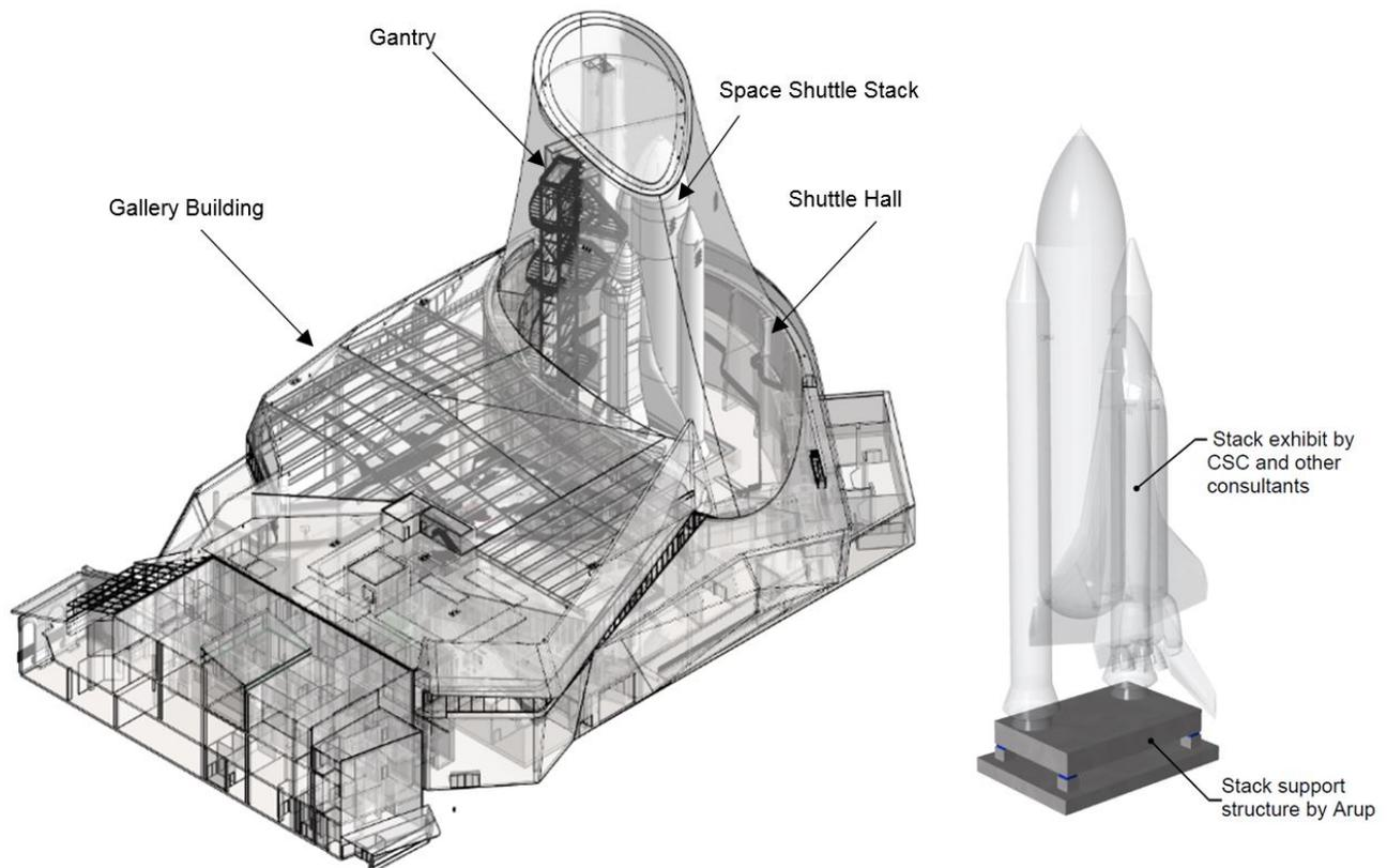
Figure 1- Stack Exhibit and Support System
