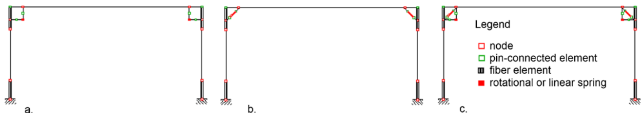
Fig. 7 – Scheme of the additional beam-to-column devices.
