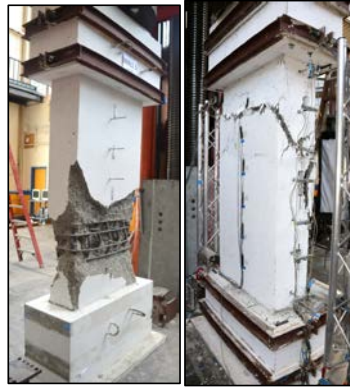
Fig. 9 – Failure mode of specimens C1, C2, C3 (left) and H1 (right).
