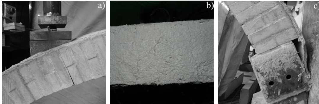
Fig. 6 – Failure details of PBO-FRCM extrados strengthened arches: a) hinge formation on the loaded cross section; b) superficial cracking of the cementitious matrix; c) shear sliding at the right abutment.
