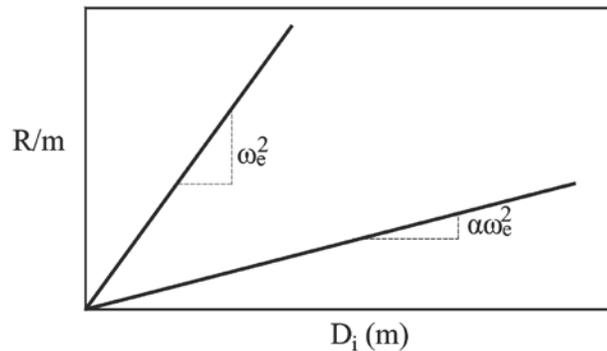
Fig. 2 Branches of the behaviour curve of the reference SDOF system.
