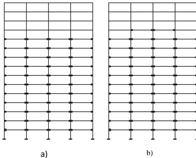
Fig. 6 Damage distribution in frame X5, a) Method proposed and b) Step-by-step analysis
