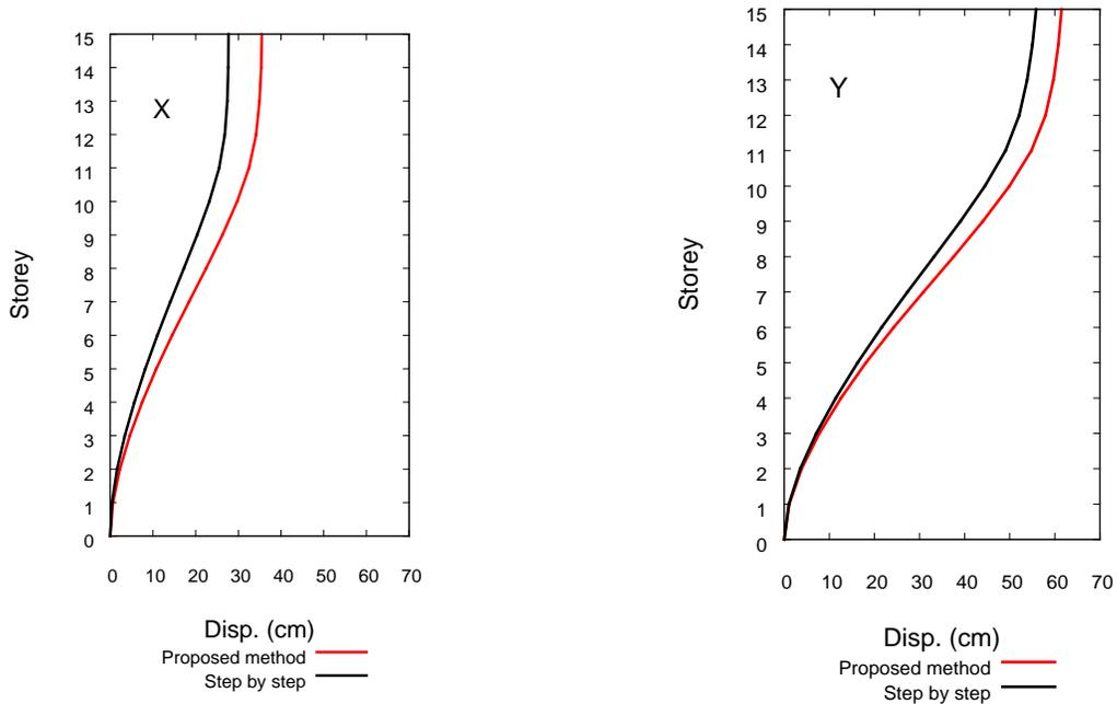
Fig. 7 Comparison of the profile of maximum horizontal displacements of frame X5
