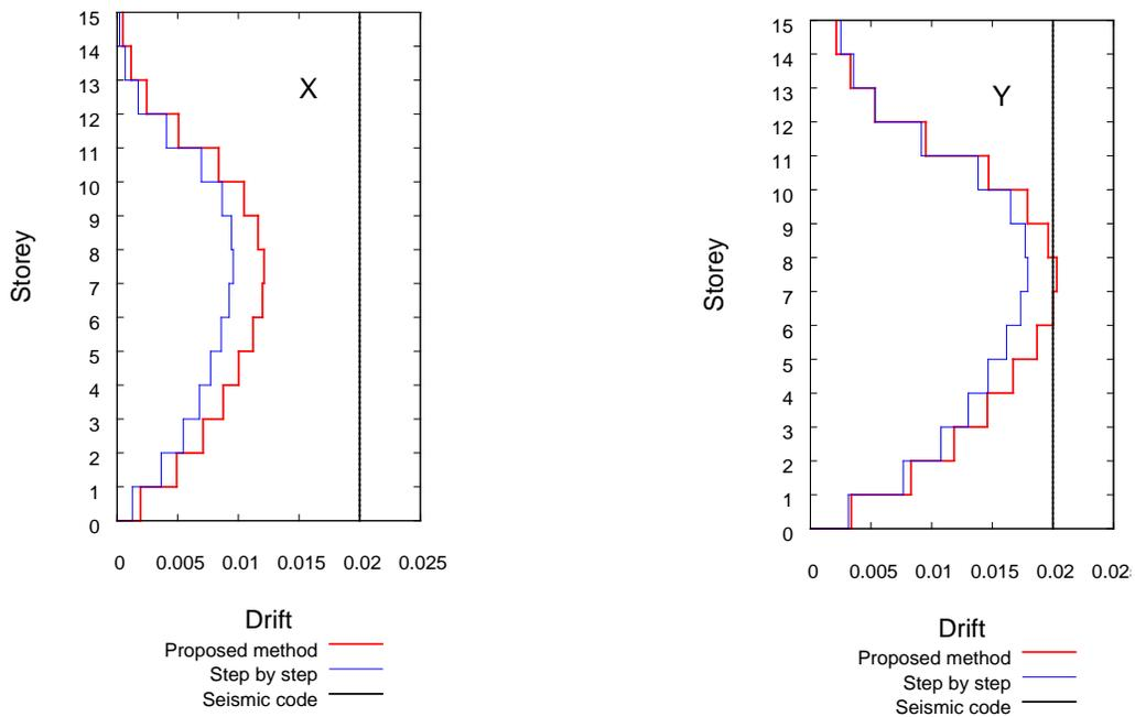
Fig. 8 Comparison of the interstorey drifts for frame X5
