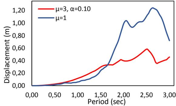
Fig. 3 Elastic and inelastic displacement spectra.
