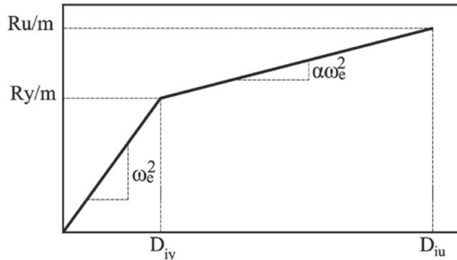
Fig. 4 Behaviour curve of a reference SDOF system.
