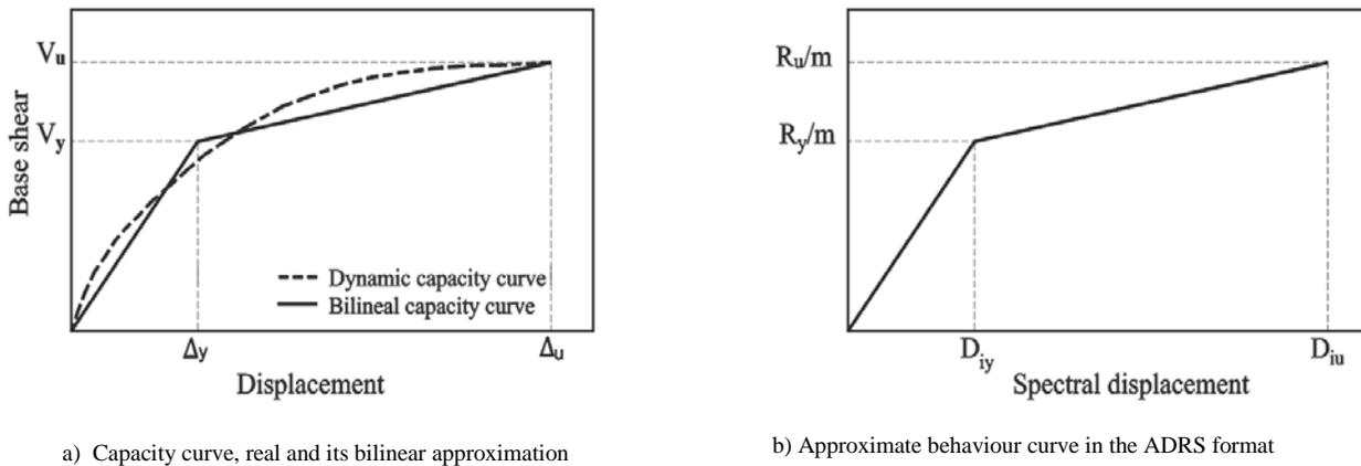
Fig. 1 Illustration of the capacity curve of a structure and the behaviour curve of the corresponding reference SDOF system as those used by the design method proposed.
