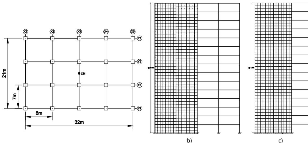
Fig. 5 Building example, a) Building plan, b) Frame Y1 and c) Frame X1.
