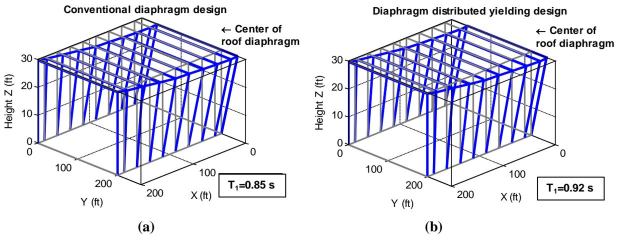
**Fig. 5: Fundamental mode shape and respective period for shaking along the short direction: (a) conventional (ASCE 7-10) diaphragm design and (b) diaphragm distributed yielding design (displacement amplification factor=40; 1ft=0.3048m)**
