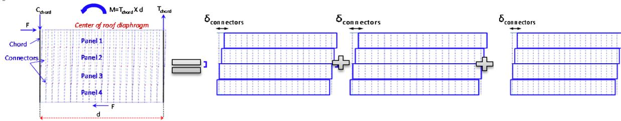
**Fig. 4: Illustrative representation of the analytical inelastic roof diaphragm model developed in MATLAB**
