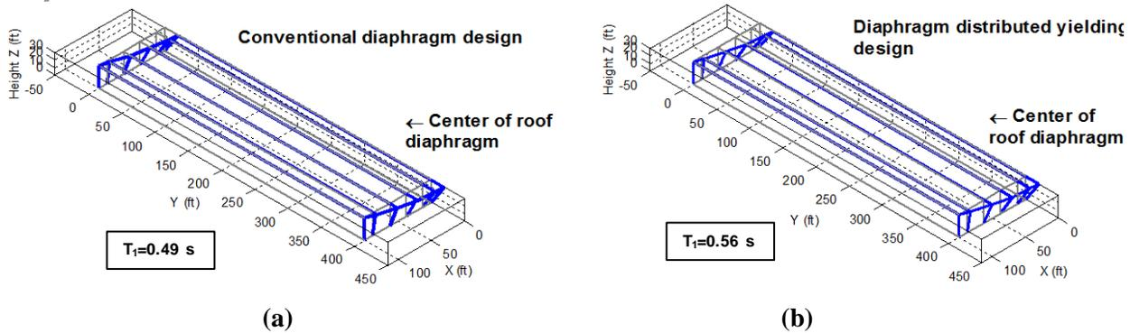
**Fig. 6: Fundamental mode shape and respective period for shaking along the long direction: (a) conventional (ASCE 7-10) diaphragm design and (b) diaphragm distributed yielding design (displacement amplification factor=20; 1ft=0.3048m)**
