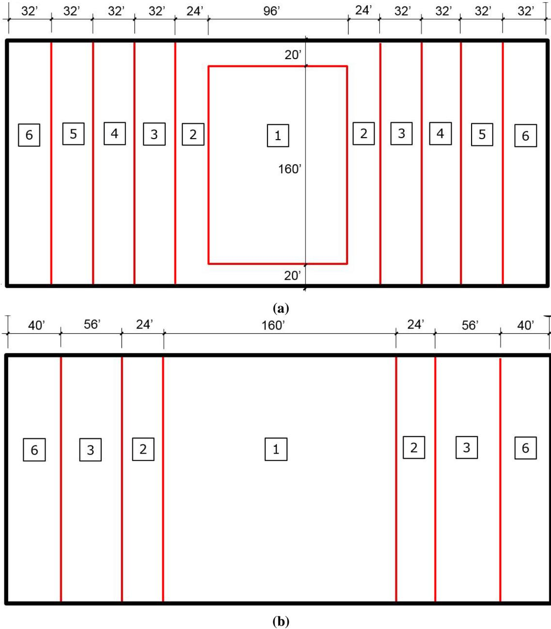
Fig. 2: Roof diaphragm nailing details for: (a) existing/conventional design of RWFD buildings and (b) design applying the distributed yielding concept (1ft=0.3048m)
