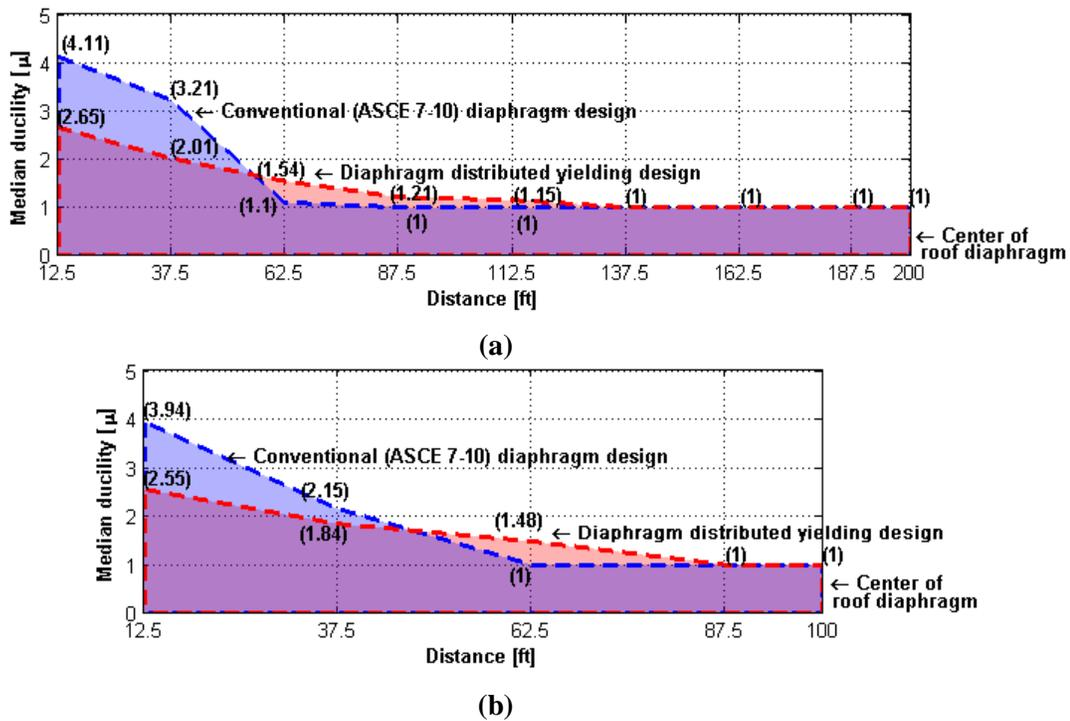
**Fig. 10: Median ductility distribution using the FEMA P695 ground motions at MCE intensity level for: (a) short direction excitation and (b) long direction excitation (1ft=0.3048m)**
