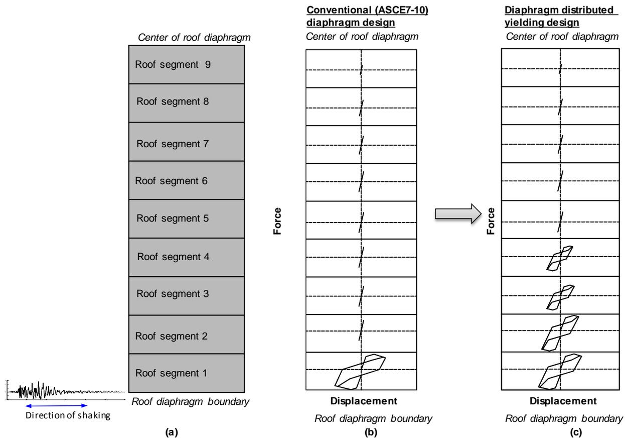
Fig. 1: Expected hysteretic response with: (a) roof discretization, (b) existing design of RWF buildings and (c) design applying the distributed yielding concept [6, 7]
