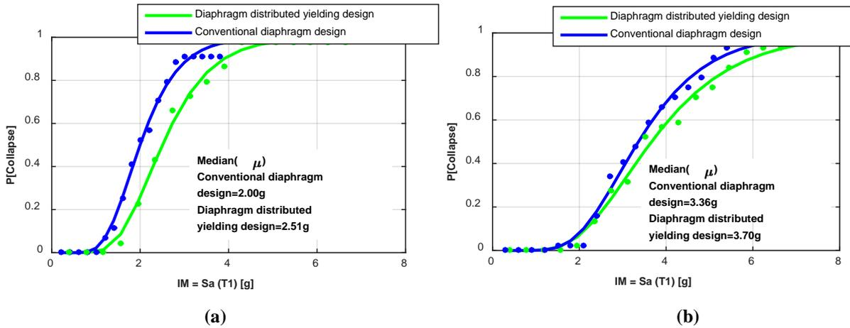
**Fig. 9: Collapse fragility curves for conventional (ASCE 7-10) and distributed yielding diaphragm design: (a) short direction excitation and (b) long direction excitation**
