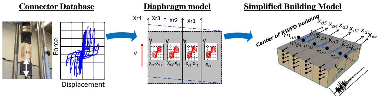
Fig. 3: Three step sub-structuring numerical framework
