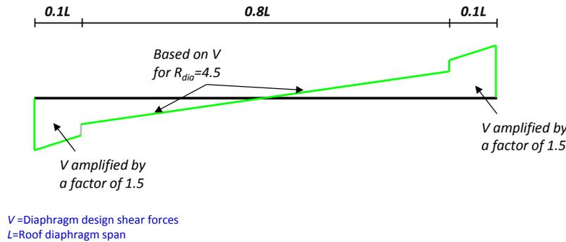
**Fig. 11: Roof diaphragm design shear forces for proposed seismic design approach to ensure distributed roof diaphragm yielding [16]**
