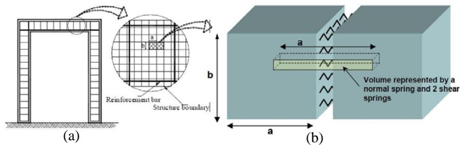
Fig. 2 – (a) Element Generation for AEM, (b) Spring Distribution and Area of Influence of springs
