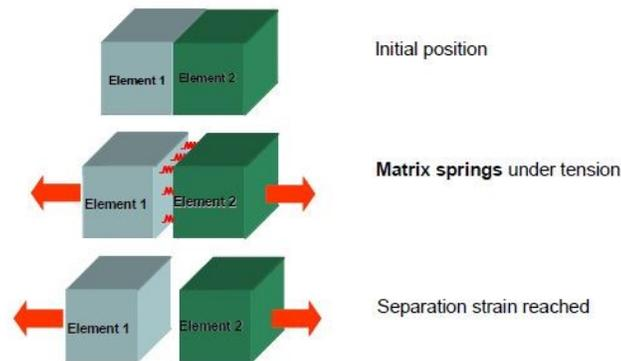
Fig. 3 – Element separation
