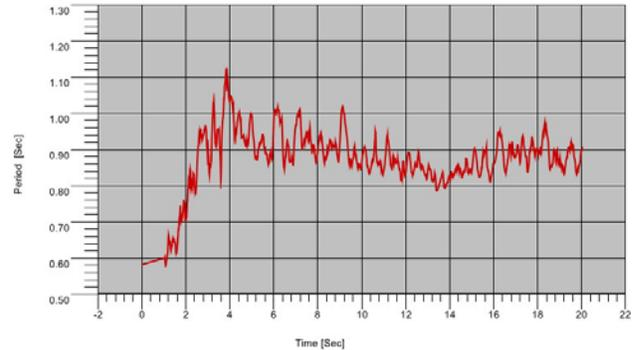
Fig. 12 – Structure period vs. time in the X (left) and Y (right) directions (67% cases)
