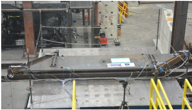
Fig. 4 –45° skew bridge model on Shake Table No.1
