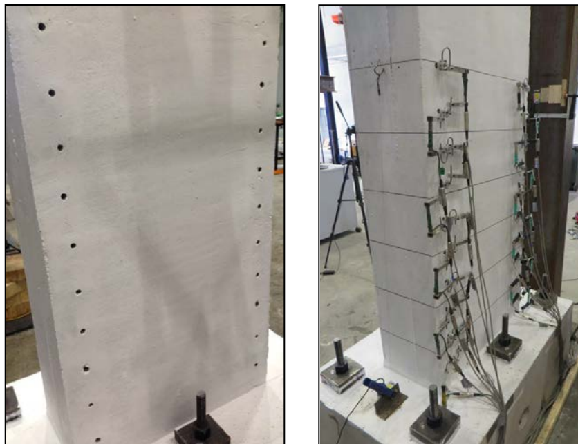
Fig.4 – Holes in cover concrete for access to threaded inserts on exterior reinforcing bars, before and after attachment of displacement gauges
