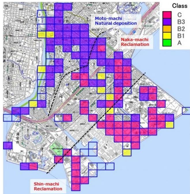
Fig.14 Hazard map for potential damage to wooden houses based on the new criterion proposed by MLIT
