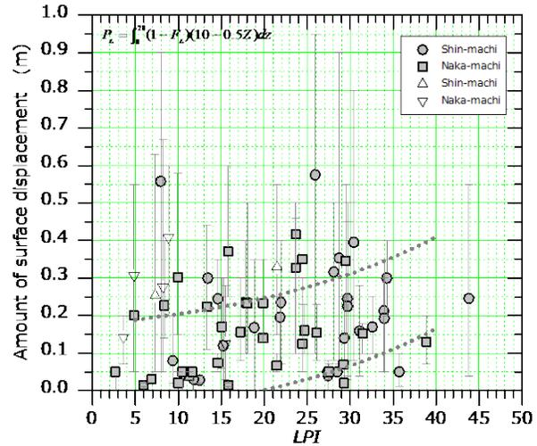
Fig.12 Relationship between *LPI* and ground displacement in Case 1-1
