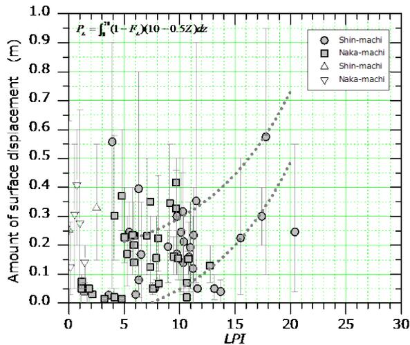
Fig.11 Relationship between *LPI* and ground displacement in Case 2-3
