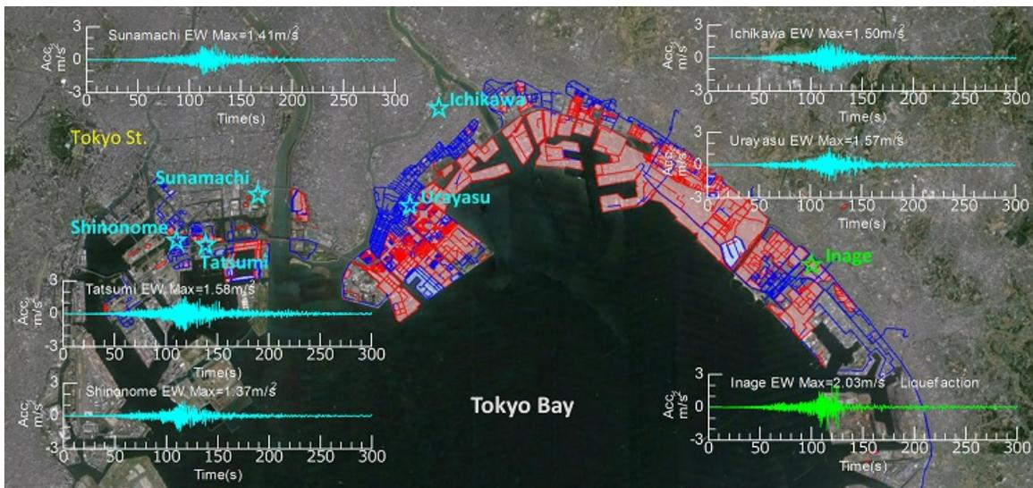
Fig.1 Liquefaction area and observed earthquake motion of the Tokyo Bay area, by K-NET
