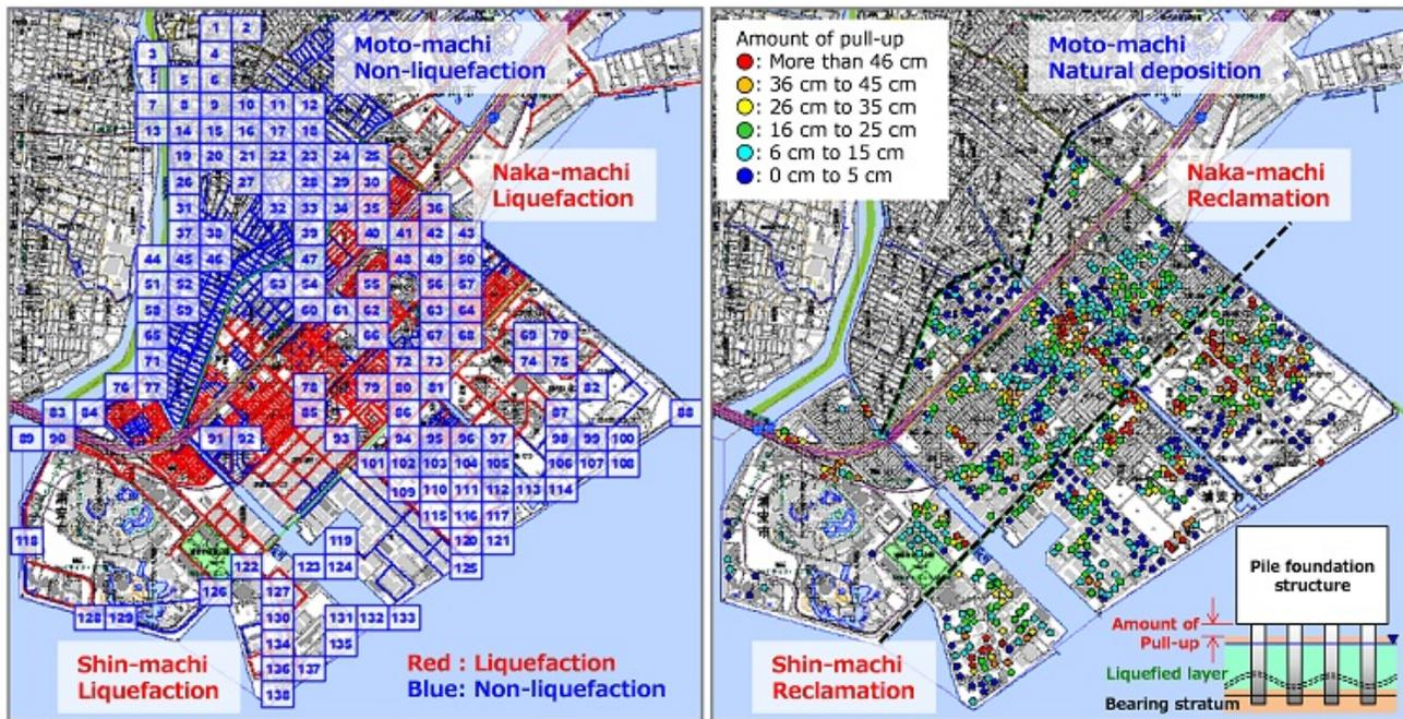
Fig.2 Meshes where RPSMs were constructed for Urayasu, and liquefaction-induced ground displacement
