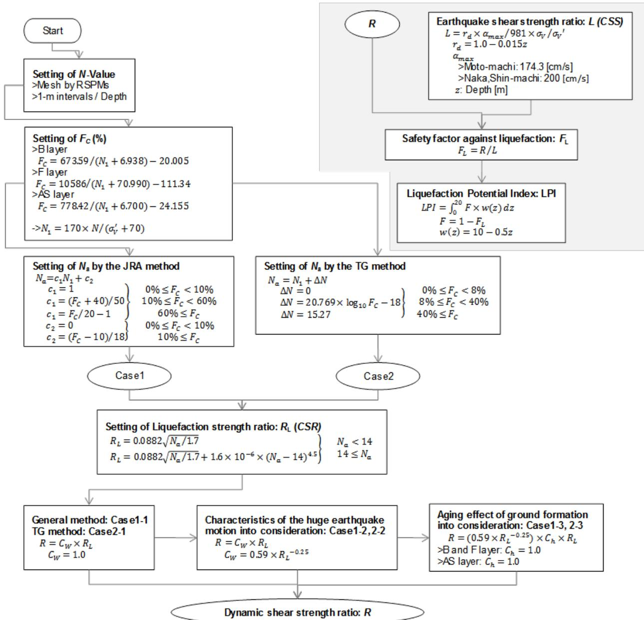
Fig.4 Flow chart of the liquefaction judgments
