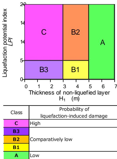
Fig.13 Probability banks for liquefaction-induced damage to houses by  $LPI$  and  $H_1$
