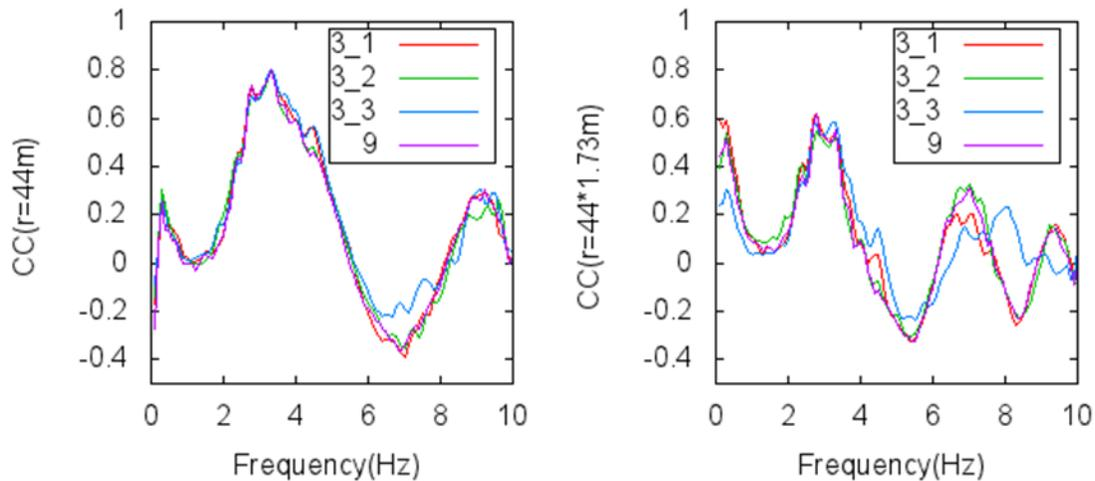
Fig.3 Spatial autocorrelation coefficients for vertical microtremors by using SPAC method. Left figure shows SPAC coefficients for a distance of 44 m and right figure shows those for a distance of 86.6 m. The figures show relation between regular triangle type array and regular nonagon type one.
