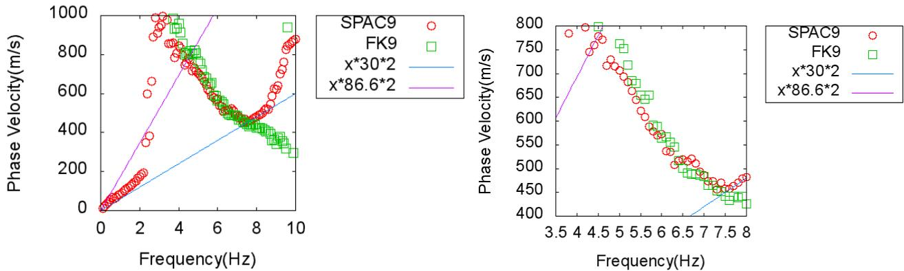
Fig. 6 Phase velocities of Rayleigh wave estimated from vertical microtremors by SPAC method and FK method. Red circles indicate phase velocities by SPAC method and green square indicate phase velocities by FK method. Left figure shows normal view. Right figure shows enlarged view. A minimum distance in the case of a regular nonagon type array is about 30 m.
