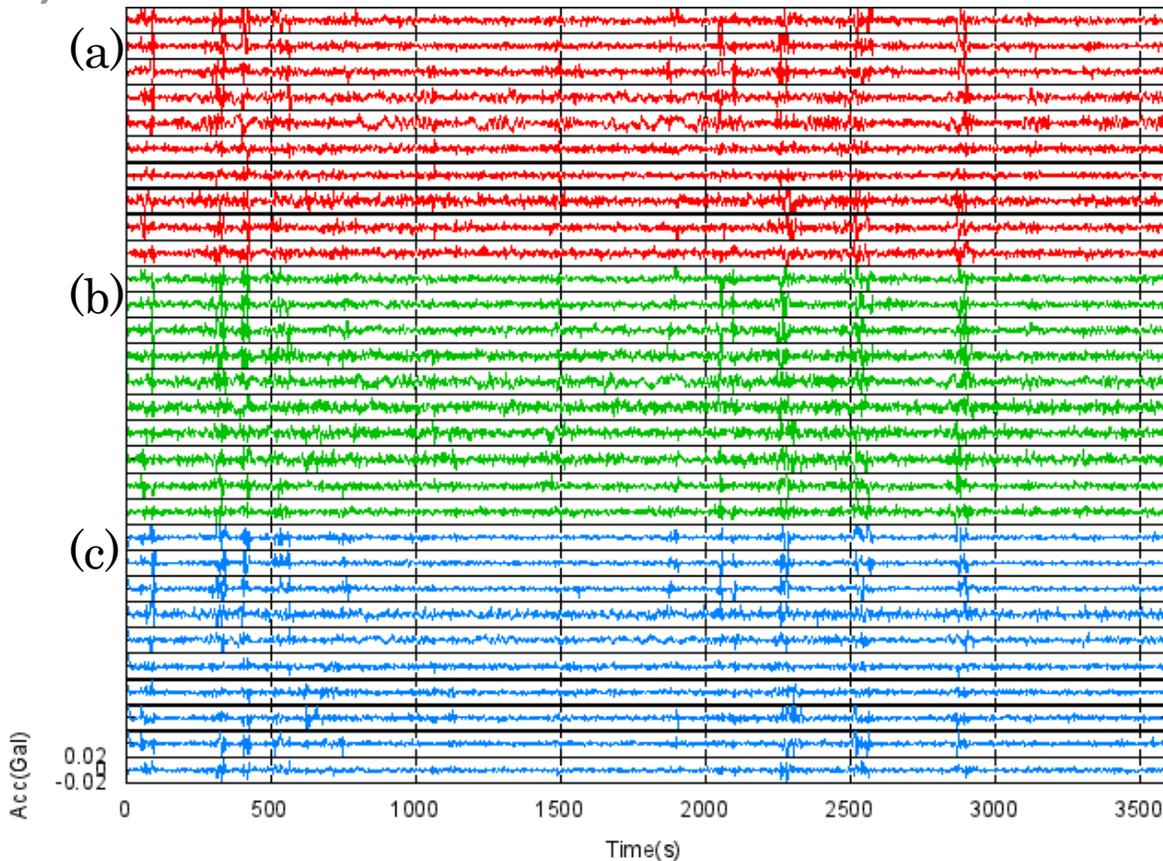
Fig. 2 Acceleration waveform of observed microtremor array records. (a) Red waveforms indicate EW component, (b) Green indicate NS component (c) Blue indicate UD component. A top waveform for each component is located at the north position. A bottom waveform for each component is located at a center.
