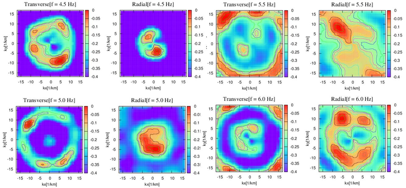
Fig. 8 F-K power spectra of horizontal microtremors at frequencies of 4.5, 5.0, 5.5 and 6.0 Hz. We can see that transverse FK power shows strong powers on a circumstance. This suggests transverse-type microtremor arrive from various orientations.
