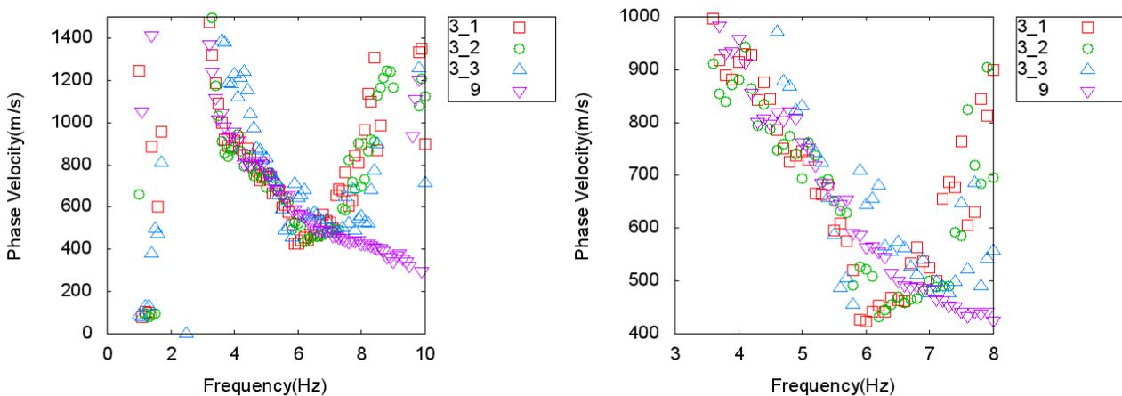
Fig. 5 Phase velocities of Rayleigh wave estimated from vertical microtremors by FK method. Left figure shows normal view. Right figure shows enlarged view. A purple inverted triangle indicate phase velocities estimated from records of the nonagon array. A red square, a green square and a blue triangle indicate phase velocities estimated from the records of the triangle arrays. A minimum distance in the case of a regular nonagon type array is about 30 m.
