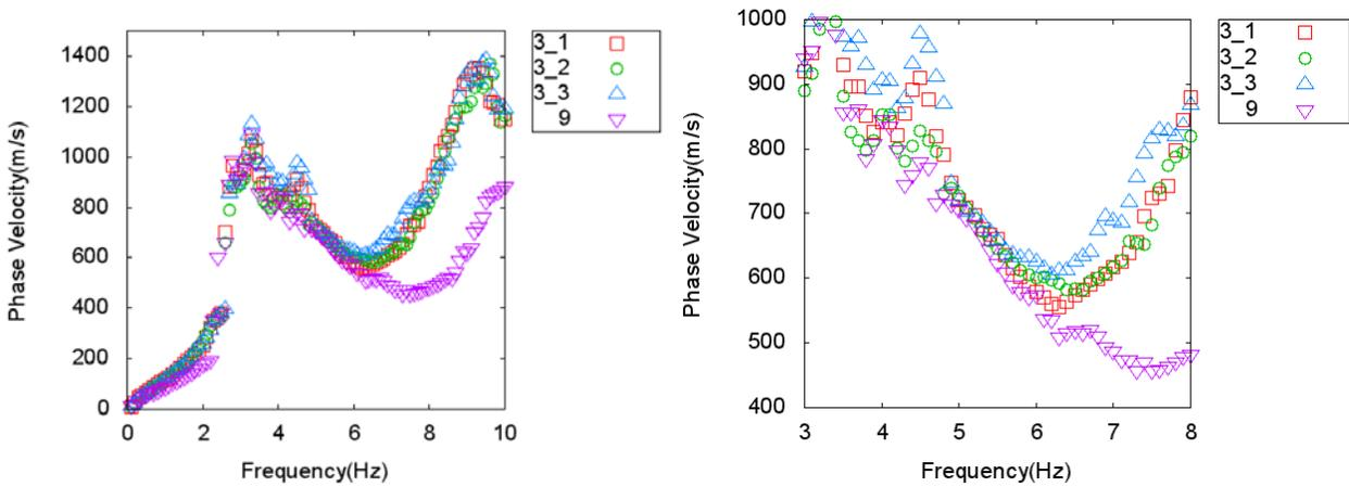
Fig. 4 Phase velocities of Rayleigh wave estimated from vertical microtremors by SPAC method. Left figure shows normal view. Right figure shows enlarged view. A minimum distance in the case of a regular nonagon type array is about 30 m.
