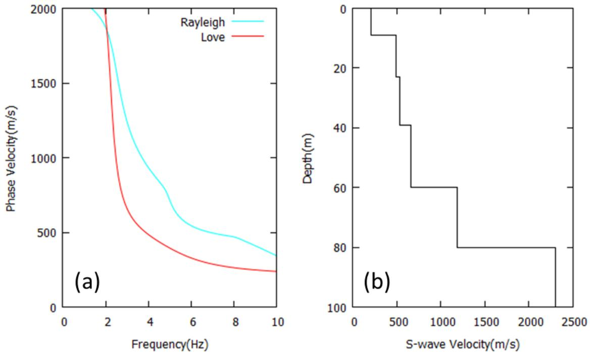
Fig.10 Phase velocities of Rayleigh and Love waves calculated from S-wave velocity structures. (a) Calculated phase velocities of Rayleigh waves. (b) S-wave velocity structure used for the calculation. S-wave velocity structure were estimated from previous studies and bore hole data in this site. It is expected that phase velocities are not the same at the frequency range in this site.
