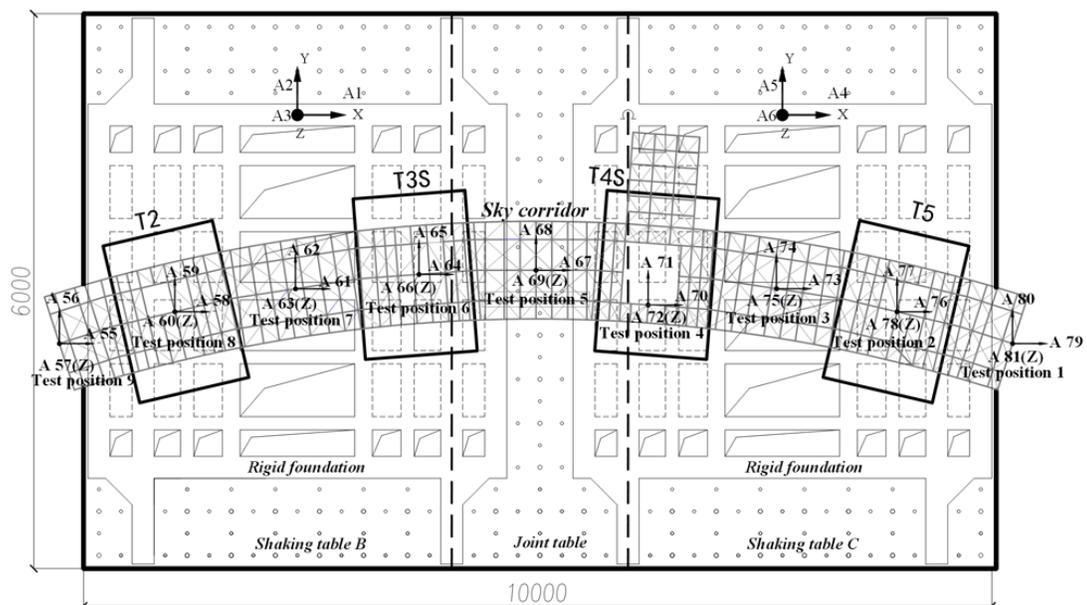
Fig. 5– Plan layout of model structure
