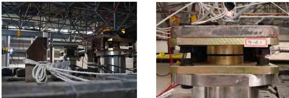
Fig. 3– scaled friction pendulum and viscous damper in the experimental model
