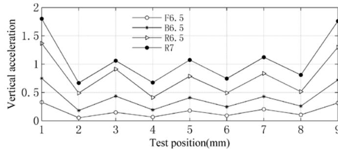
Fig. 10–Vertical acceleration of sky corridor under different earthquake level
