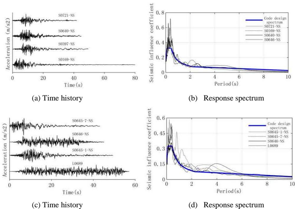
Fig. 6 – Input seismic waves and response spectrum.
