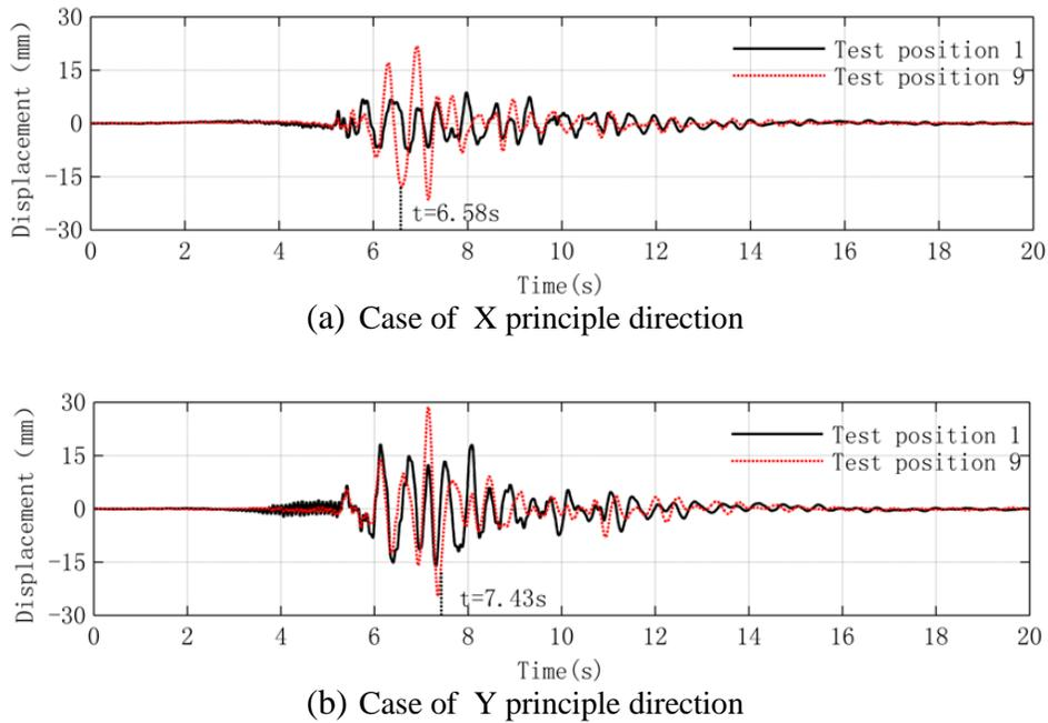
Fig. 9–Displacement time history of sky-corridor under rare earthquake of intensity 7
