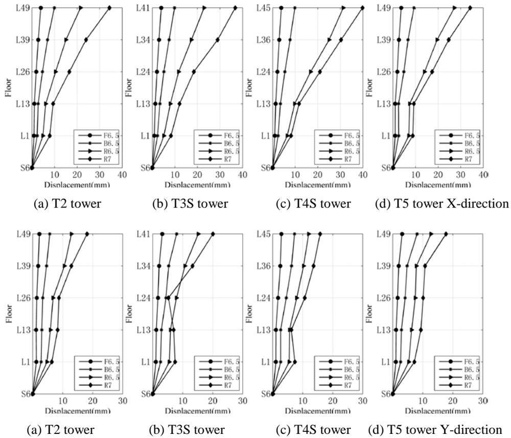
Fig. 8–Distribution of max displacements of towers
