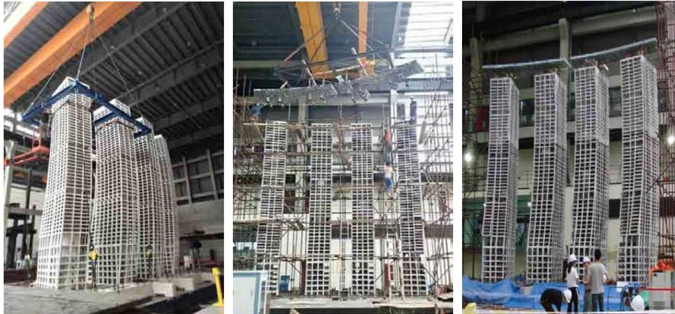
Fig. 4– Installation of four towers and shy-corridor
