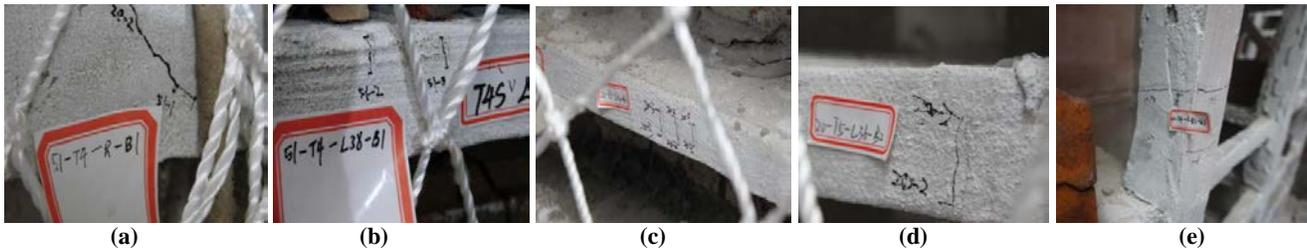
Fig. 7–Failure patterns under major earthquakes of intensity 7: (a) beam at the top floor of T4S tower; (b) beam at the 38 th floor of T4S tower; (c) beam at the 34th floor of T5 tower; (d) beam at the 36th floor of T5 tower; (e) column at the 12th floor of T5 tower
