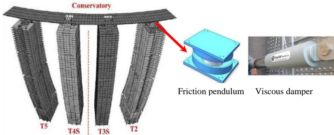
Fig. 1 –Overall structure of building
