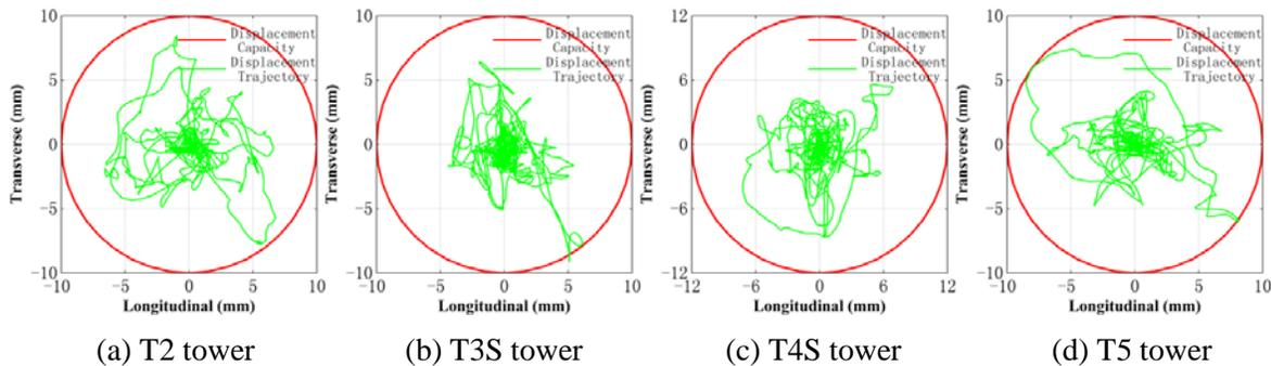
Fig. 11–Movement orbit of each Tower’s bearing under 7 major levels
