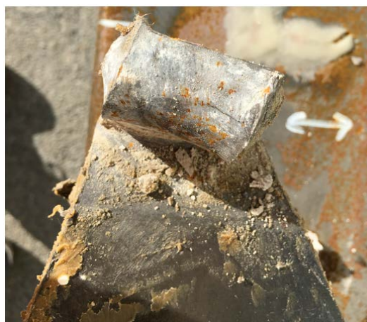
Fig. 6 – Yielding core fracture and fold onto transition region
