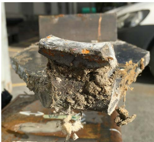
Fig. 6 – Yielding core fracture and fold onto transition region
