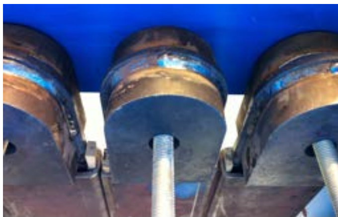
Fig. 3 – BRB specimen vertical suspension
