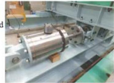
Fig. 4 – Inertial mass damper
