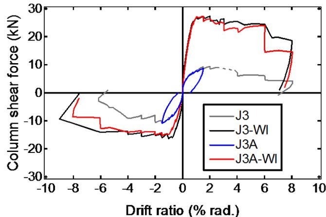
Fig. 11 – Skeleton curves of the hysteresis loops in Fig. 10
