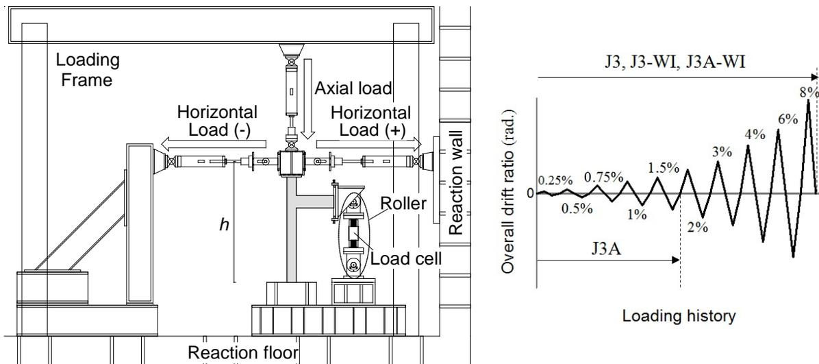
Fig. 8 – Test setup and horizontal loading history
