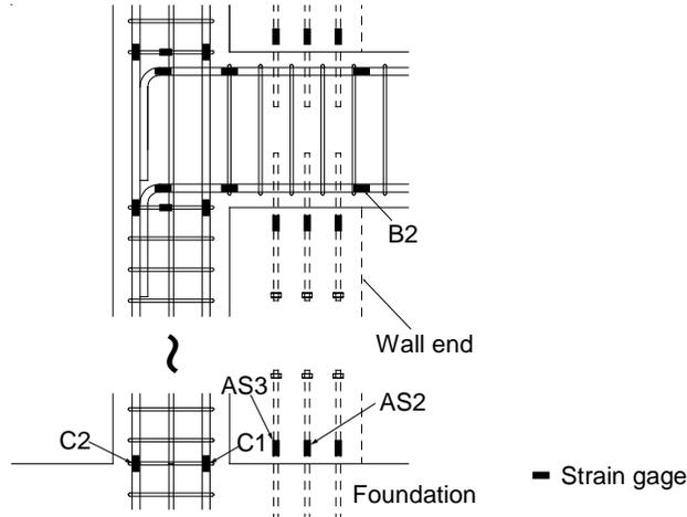
Fig. 9 – Strain gauge arrangement
