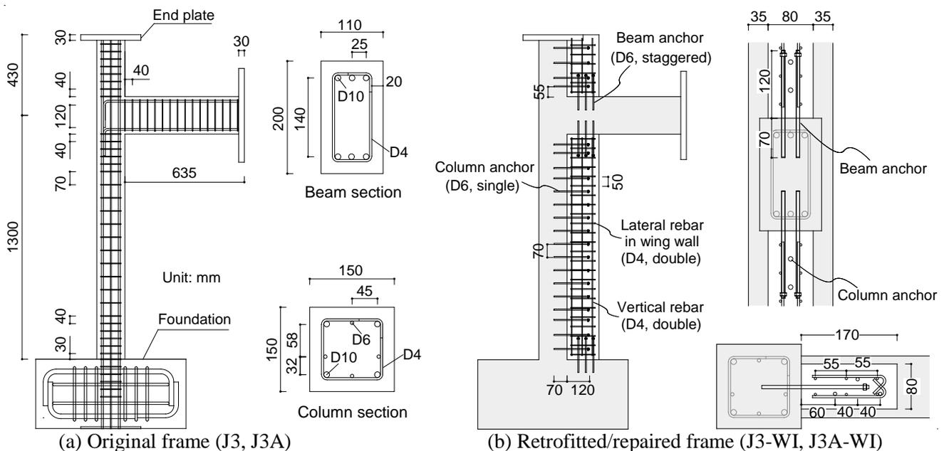
Fig. 7 – Dimensions and reinforcement details of the specimens
