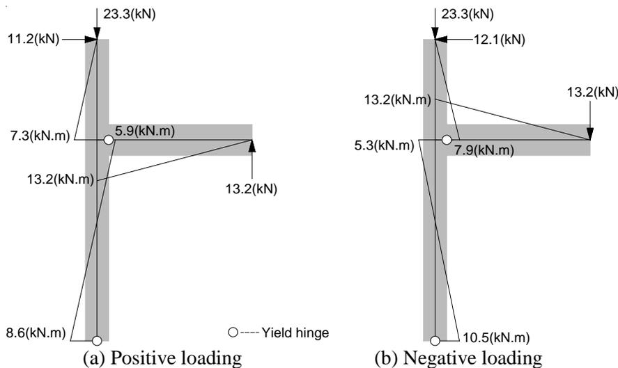
Fig. 15 – Moment diagrams upon the ultimate failure mechanism estimated for the benchmark specimen J3
