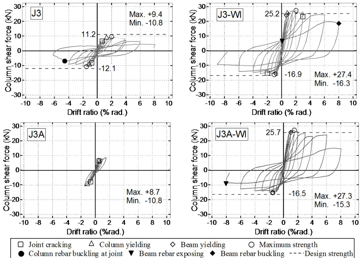
Fig. 10 – Horizontal load-drift relationships
