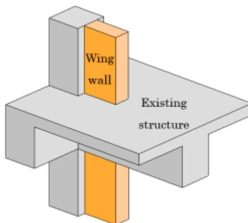
Fig. 1 – Proposed retrofitting/repairing method by installing RC wing walls
