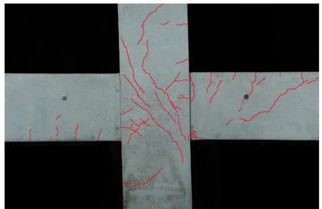
(c) Story drift angle 1/33 [rad] (the first cycle in the positive direction)
