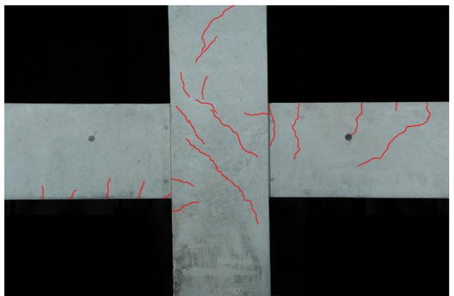
(b) Story drift angle 1/50 [rad] (the first cycle in the positive direction)
