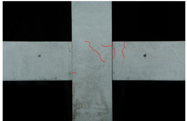
(a) Story drift angle 1/100 [rad] (the first cycle in the positive direction)
