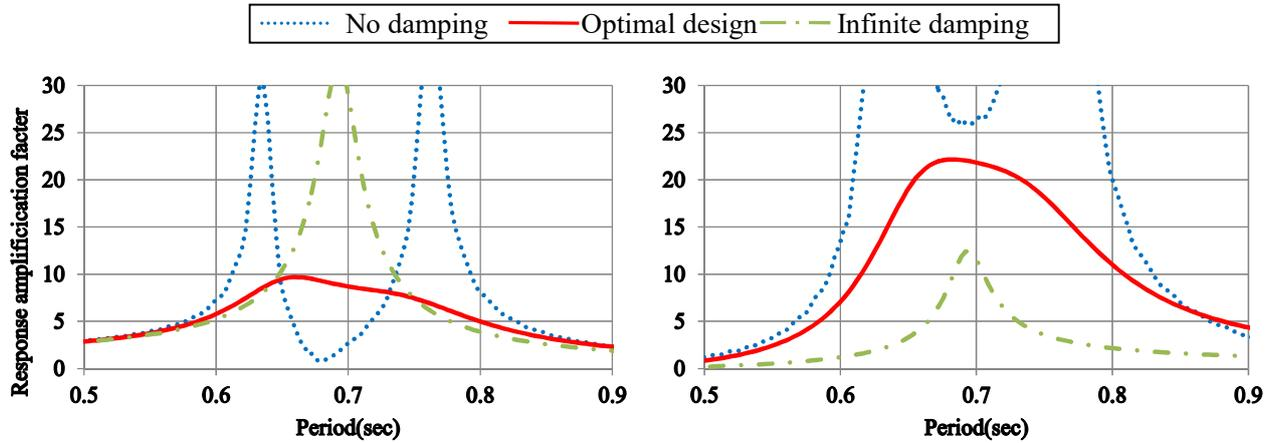
Fig. 4-1—Response amplification factor of DM outside frame coupling vibration control model
