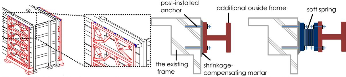
Fig. 1-1—DM outside frame coupling vibration control system
