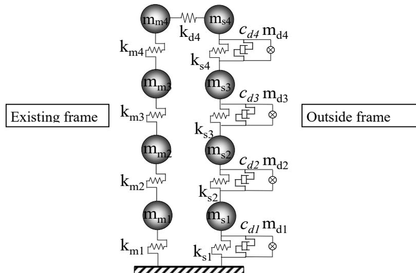
Fig. 3-1—DM Outside Frame Coupling Vibration Control model
