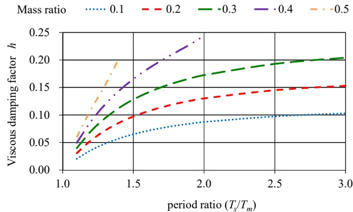
Fig. 2-3—Damping factor–period ratio relationship by mass ratio
