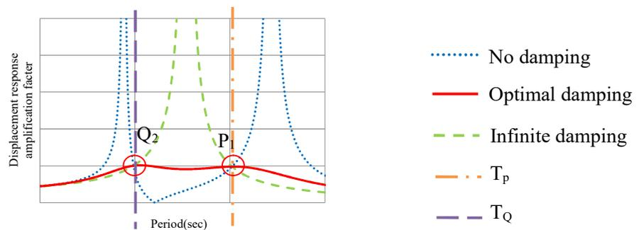
Fig. 2-2—Displacement response amplification factor curve for existing frame
