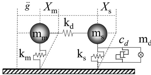
Fig. 2-1—DM outside frame coupling vibration control model
