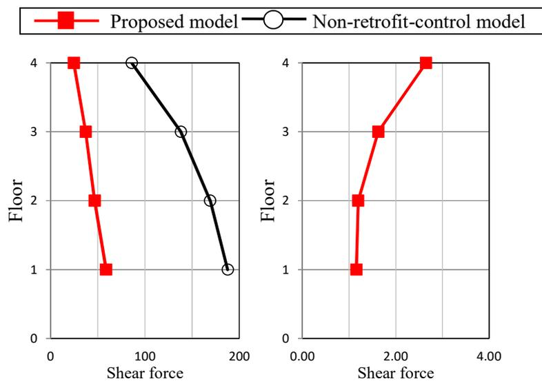
Fig. 4-2—Time history response analysis results (maximum shear force  $Q$  (kN))
