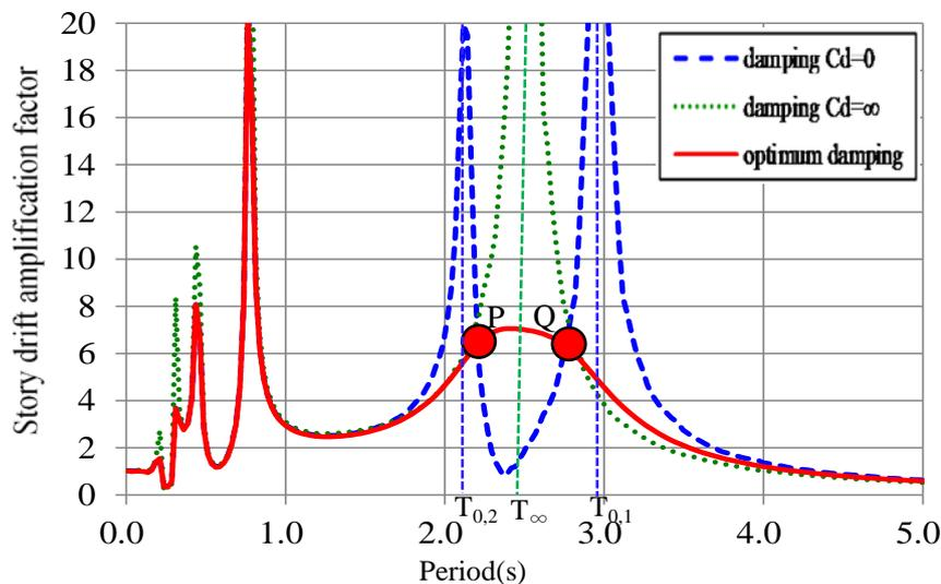
Fig. 13 – Resonance curve for the uppermost section of the tower
