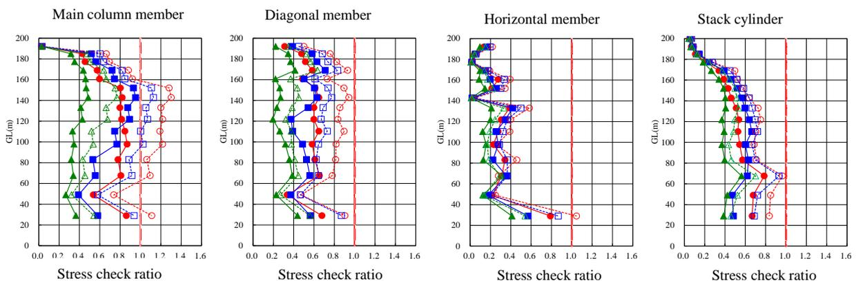
Fig. 12 – Stress check ratio (standard case)
