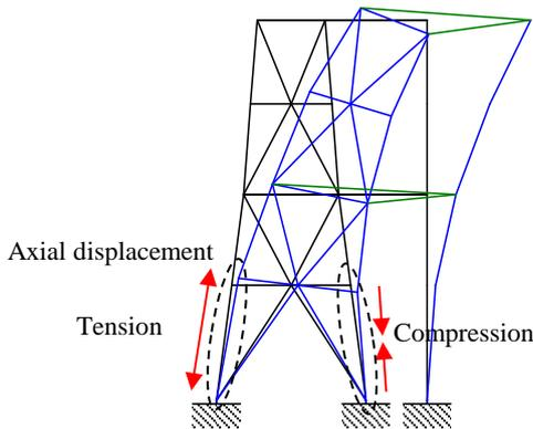
Fig.2 – Deformation mode of bending-prone structure
