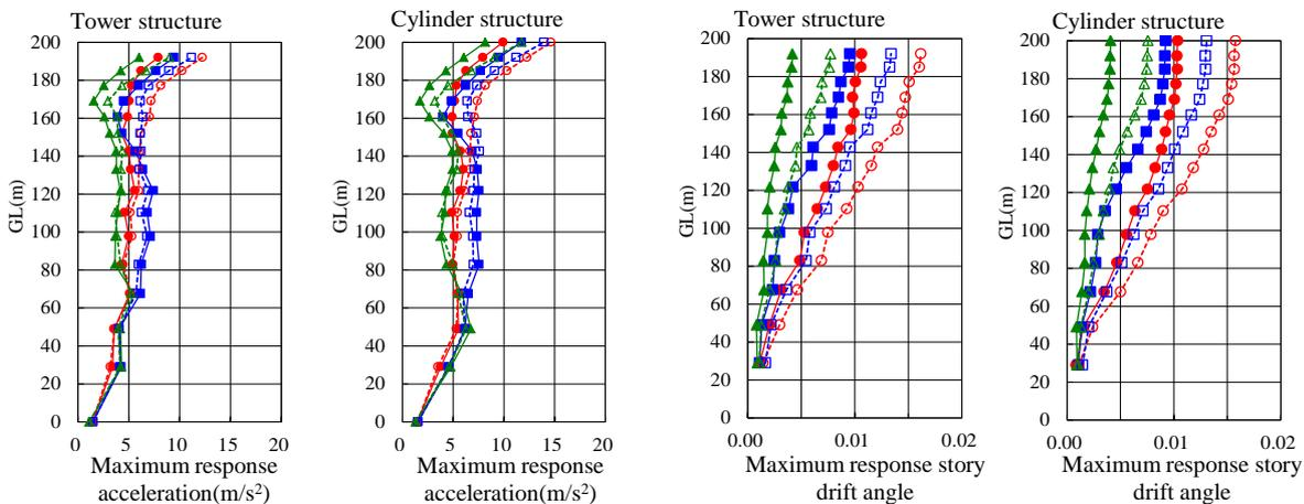
Fig. 11 – Results of 45-degree response analysis (standard case)
