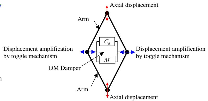
Fig.3 – Configuration of pantograph-type response control system
