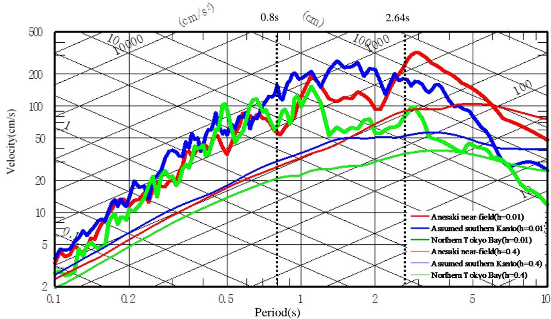
Fig. 5 – Pseudo velocity response spectrum of input ground motion
