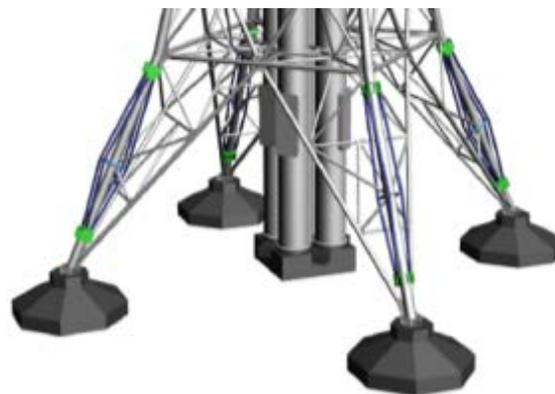
Fig. 4 – Installation of pantograph-type response control system
