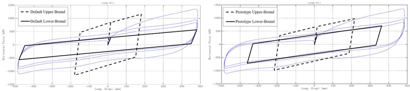
Fig. 6 – Comparison of default and prototype bounds to LR 1 test data for LR bearings
