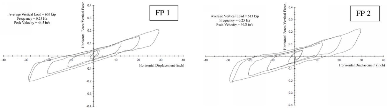
Fig. 4 – Dynamic test data of two prototype FP bearings
