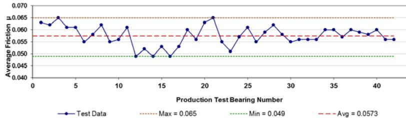
Fig. 5 – Three-cycle average  $\mu$  of 42 production FP bearings under 300kip load
