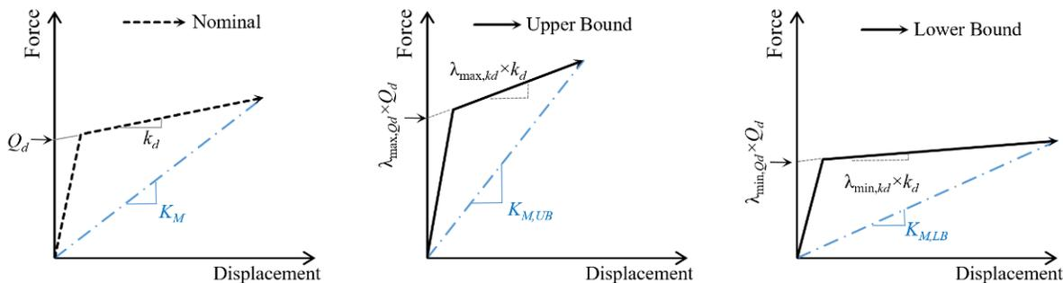
Fig. 1 – Illustration of the property modification approach to bilinear bearing model
