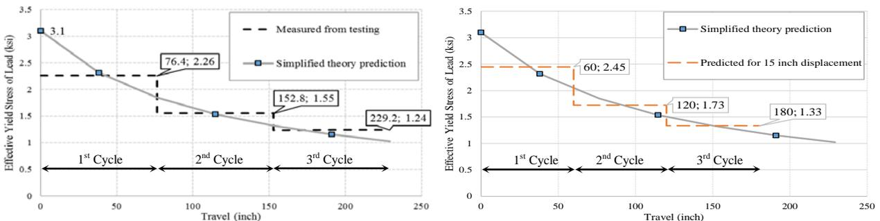
Fig. 3 – (a) Application of heating theory to test data (b) Prediction of strength for another project ( $D_M=15\text{inch}$ )
