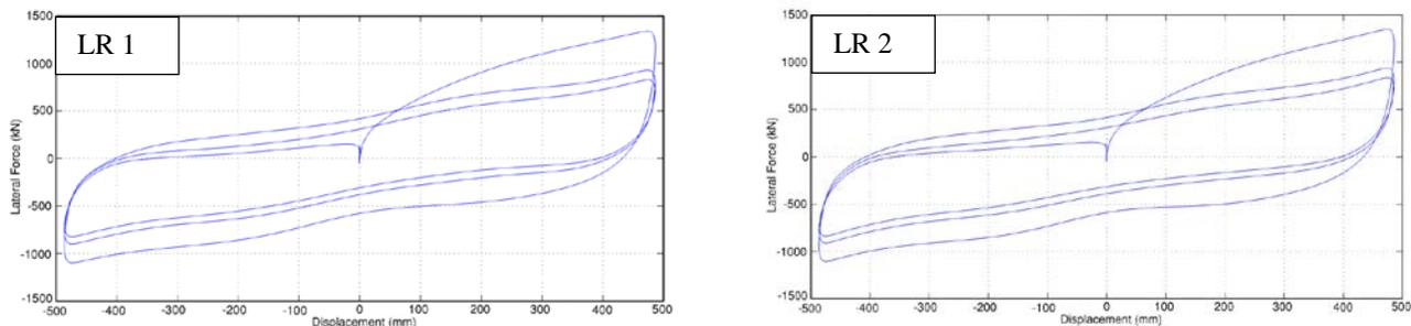
Fig. 2 – Dynamic test data of two prototype LR bearings (1inch = 25.4mm, 1kip = 4.45kN)
