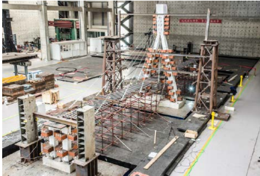
Fig. 4 Assembled bridge model
