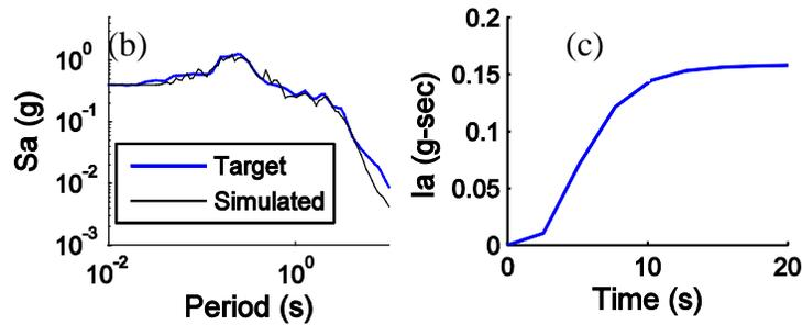
Fig. 10 –Acceleration, velocity and displacement time histories of the simulated ground motion, (b) Target and simulated spectral acceleration and (c) Arias intensity build-up.
