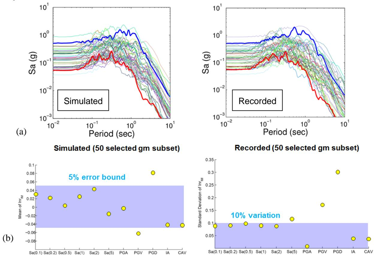
Fig. 5 – Selected 50 simulated and recorded ground-motion pairs for oscillator analyses. (a) Comparison of spectral accelerations, and (b) mean and standard deviation of IM residuals.
