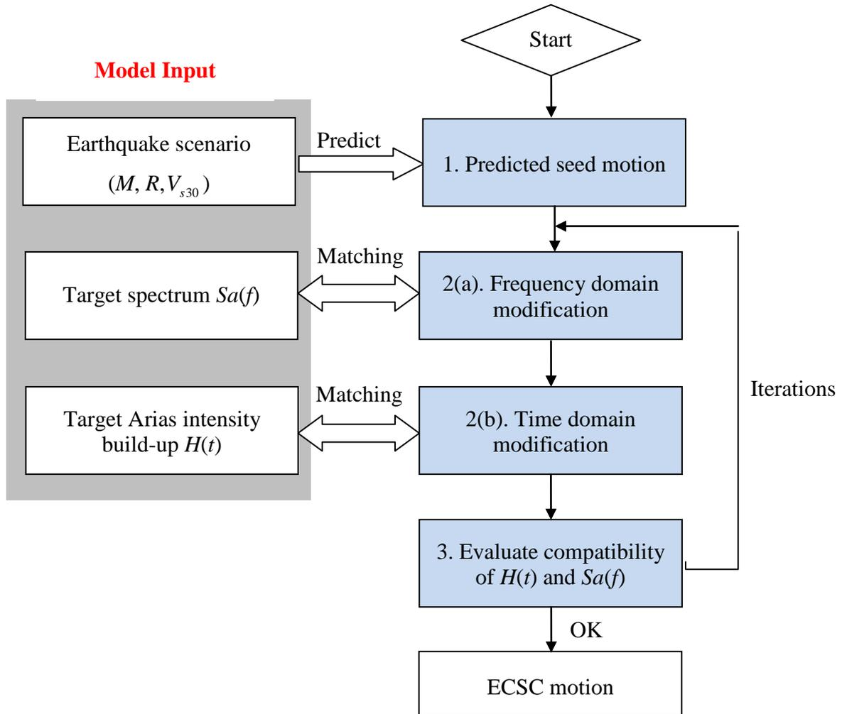
Fig. 3 – Illustration of the ECSC simulation and modification algorithms
