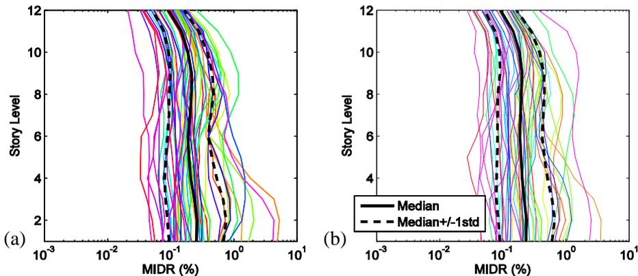
Fig. 7 – Distribution of the story-by-story MIDRs using (a) NGA dataset and (b) ECSC dataset
