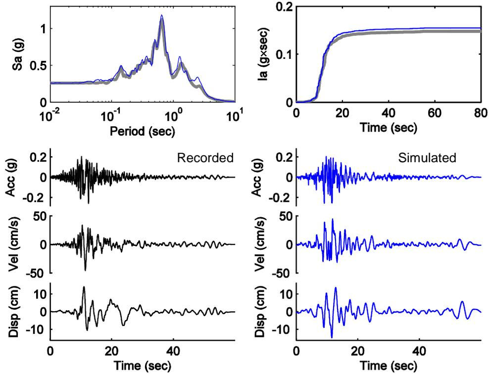
Fig.4 – Comparison of time histories, response spectra and Arias intensity build-up for the ground motion recorded at the Foster City during the Loma Prieta earthquake from the ECSC dataset and NGA dataset
