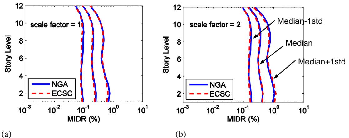
Fig. 8 – Summary of the story-by-story MIDRs using NGA and ECSC dataset with (a) scale factor = 1, and (b) scale factor = 2.
