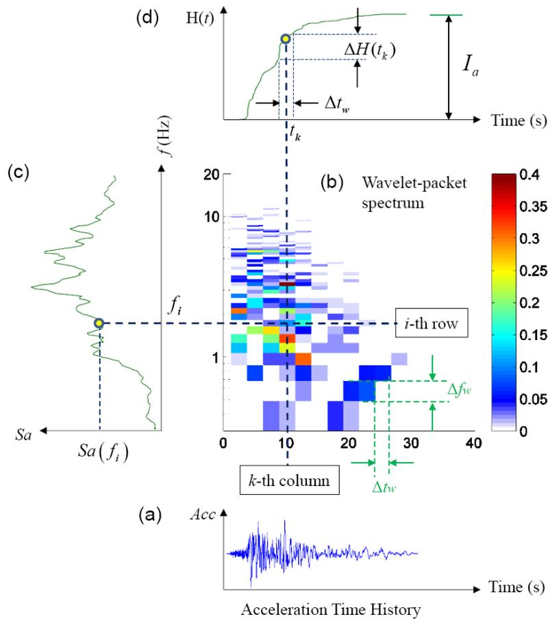
Fig. 1- Wavelet-packet spectrum, showing the distribution of squared wavelet-packet coefficients of the recorded acceleration time history at the San Valley – Roscoe Blvd station in the 1994 Northridge earthquake.
