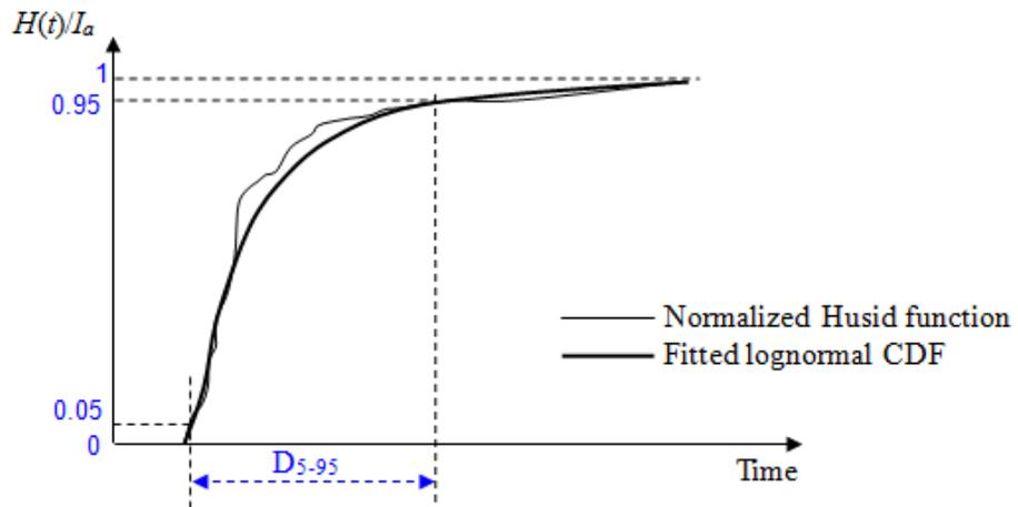
Fig. 2 – Normalized Husid function and fitted lognormal CDF
