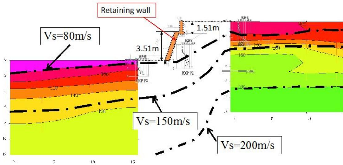
Fig. 7– Results of surface wave tests (cross section of the wall and background)
