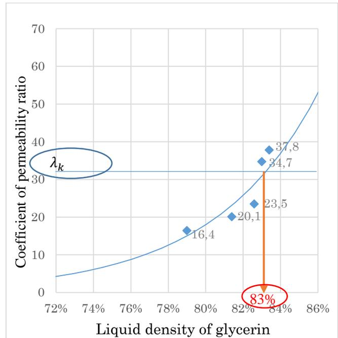
Fig. 5 – Relationship between Liquid density of glycerin and coefficient of permeability ratio
