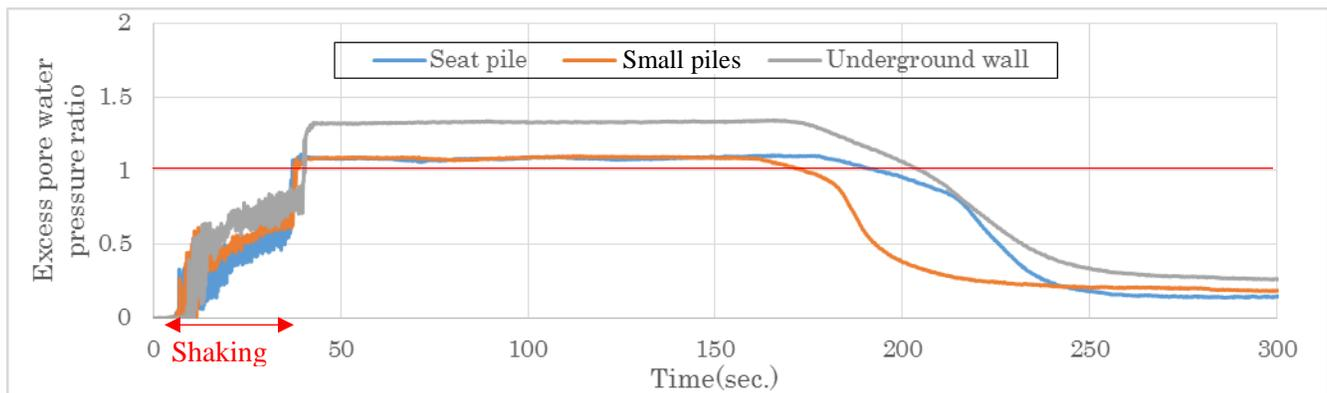
Fig. 13 – Measured results of pore water pressure at P-2 in the Fig.11
