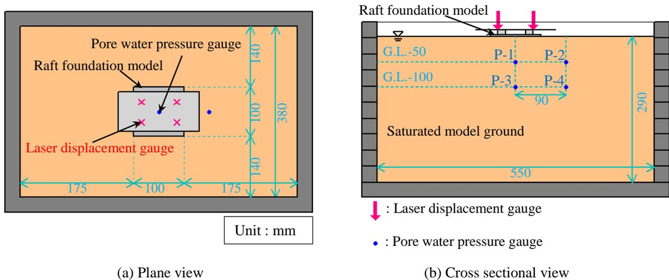
Fig. 9 – Model ground of preliminary experiment
