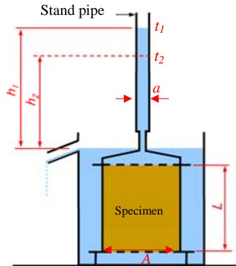
Fig. 3 – falling head permeability test
