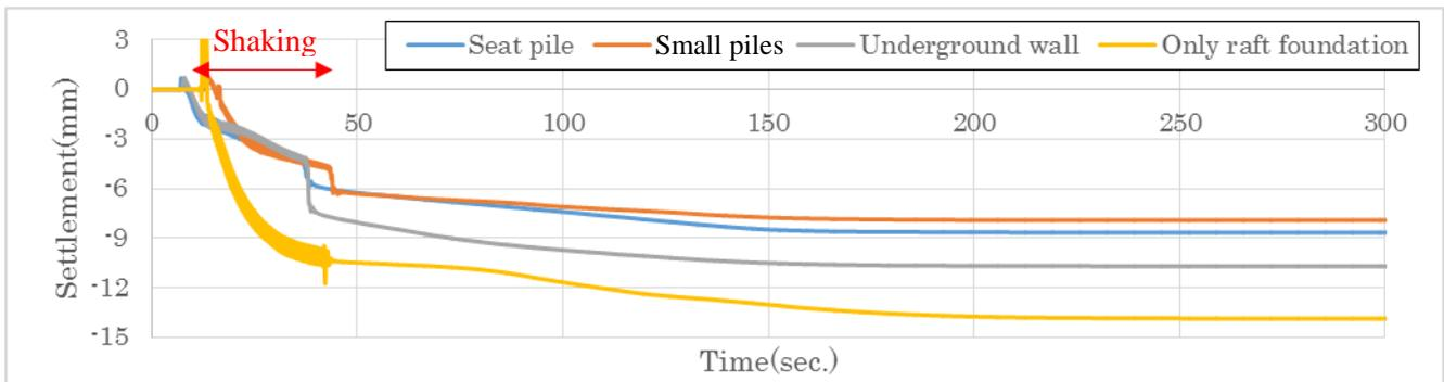
Fig. 14 – Measured results of settlement of raft foundation
