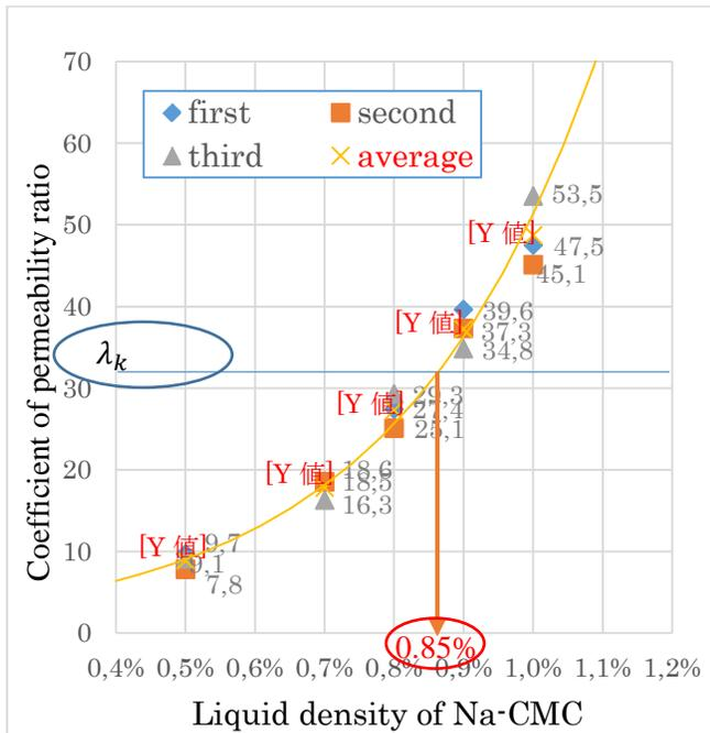
Fig. 4 – Relationship between Liquid density of Na-CMC and coefficient of permeability ratio
