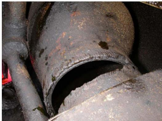
Fig. 2 – Pipe fractured by tsunami in Sendai City, Miyagi Prefecture. (Image taken by Dr. Haruki Nishi of NRIFD on June 6, 2011.)
