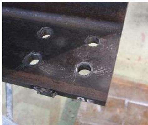
Fig. 14 – Damage of the flange in 310UC118 section
