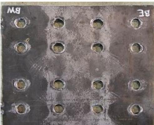
Fig. 13 – Damage in flange splice plate
