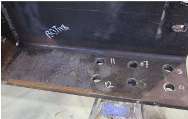
Fig. 18 –Damage of the flange in 310UC118 section
