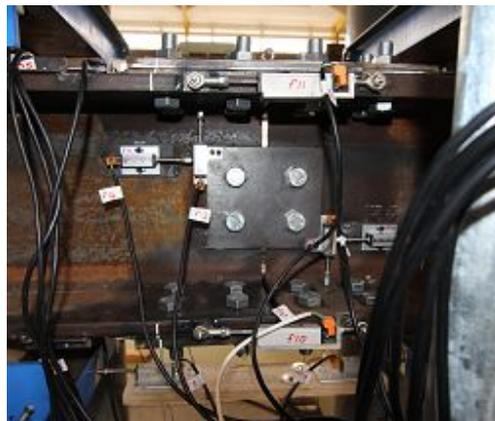
Figure 3 – Instrumentation of the connection
