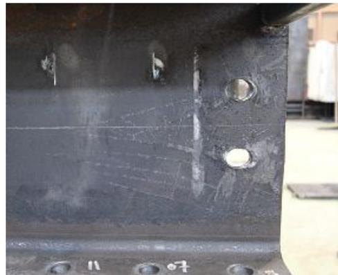
Fig. 19 –Damage of the web in 310UC118 section
