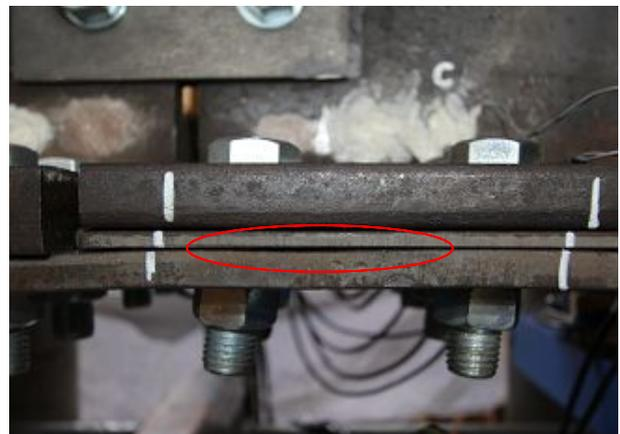
Fig. 10 – Gap between the connection plates
