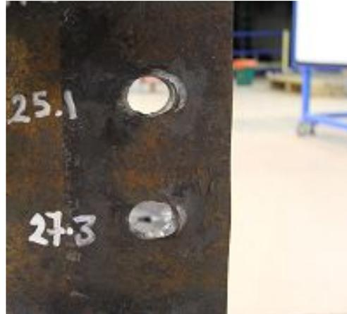
Fig. 8 – Damage of the web in 310UC118 section
