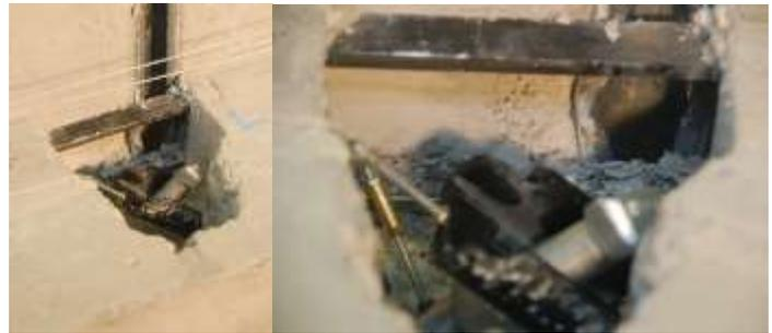
Fig. 11 Cyclic response of cantilever connections and the typical type of failure
