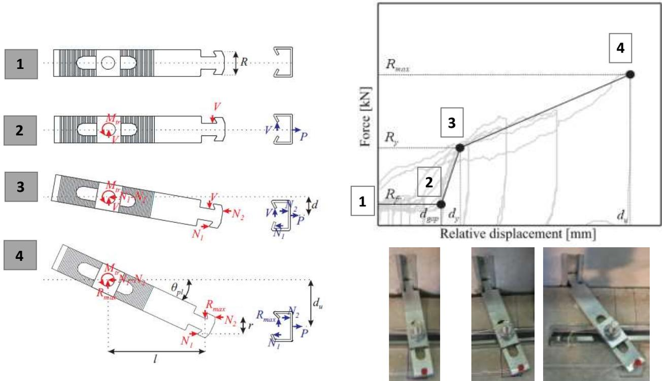
Fig. 7 The response mechanism of the hammer-head strap connections
