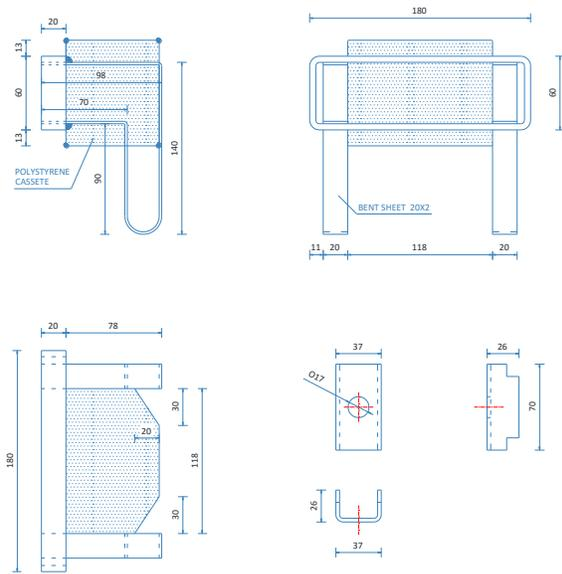
Fig. 6 The cantilever connections
