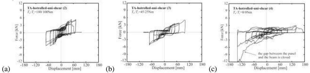
Fig. 9 The influence of the tightening torque  $T$  to the response: a)  $T = 45$  Nm, b)  $T = 180$  Nm, c)  $T = 0$  Nm
