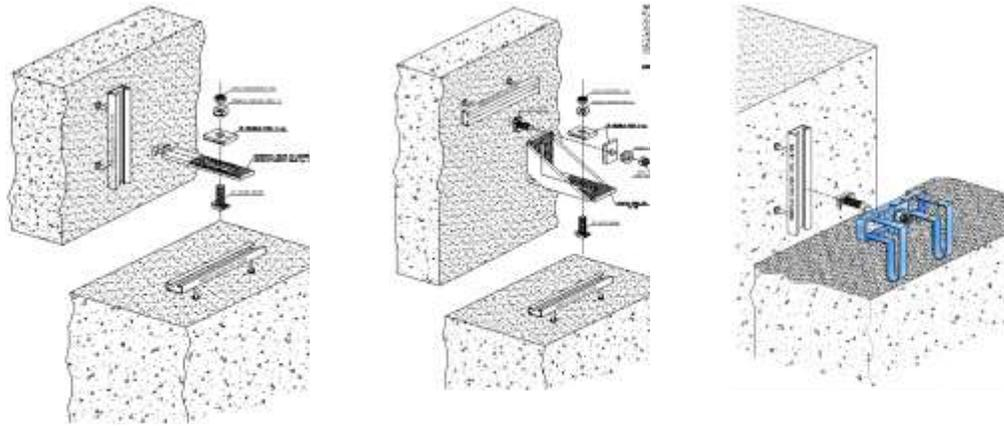
Fig. 1 Typical connections of cladding panels: a) Hammer-head tie connections, b) Angle connections, c) Cantilever connections
