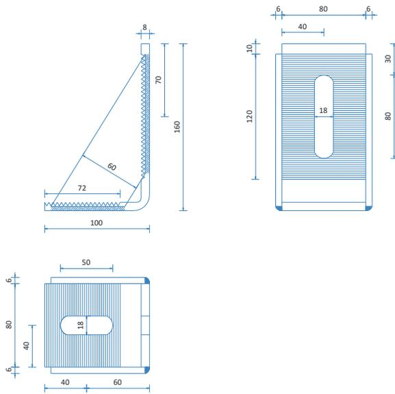
Fig. 5 The angle connection
