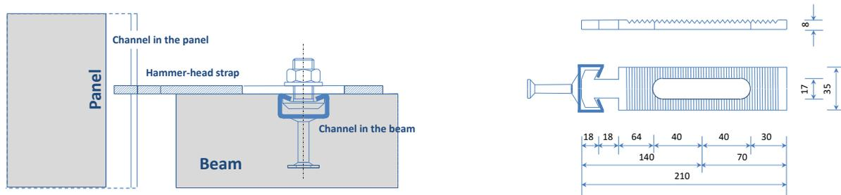
Fig. 4 The hammer-head strap connection
