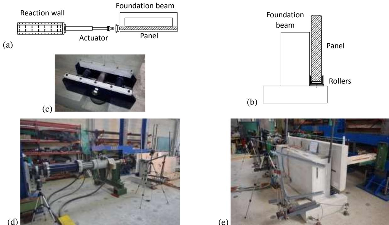
Fig. 2 Set-up of the tests: (a) plane-view, (b) side-view, (c) roller bearings, (d) the actuator, connected to the panel, (e) side-view of the test set-up
