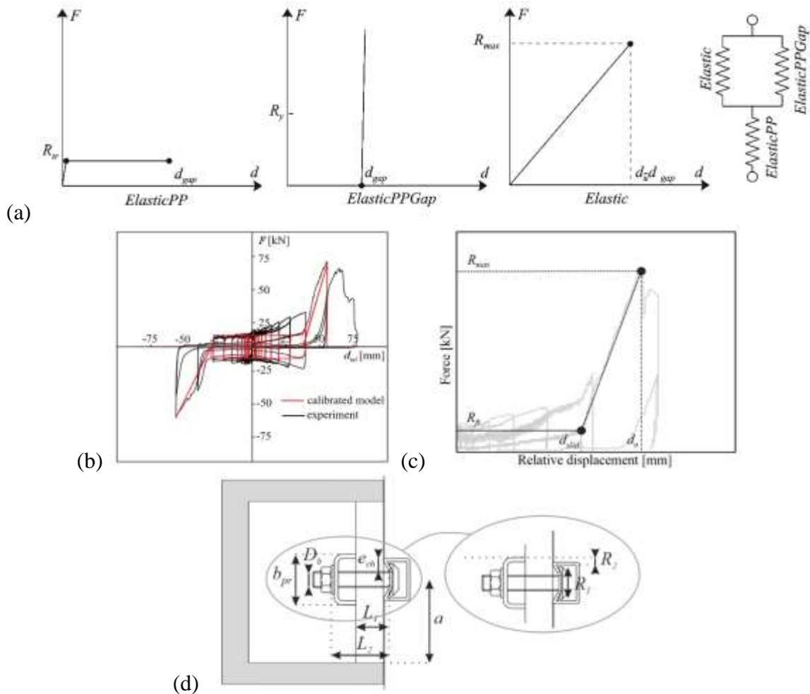
Fig. 14 Cyclic response of cantilever connections: a) the numerical model, b) the hysteretic response, c) characteristic points of the envelope, d) geometric properties, used to define the strength of the connection
