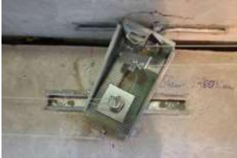
Fig. 10 Cyclic response of angle connections and the typical type of failure
