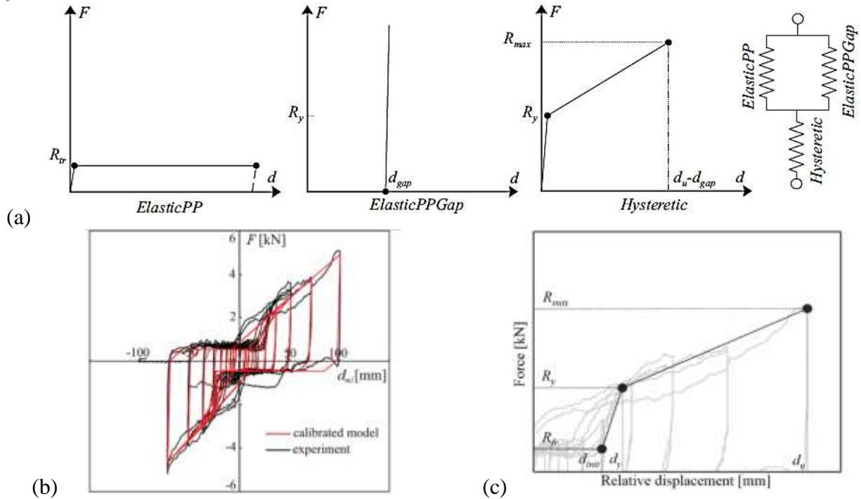
Fig. 12 Cyclic response of hammer-head strap connections: a) the numerical model, b) the hysteretic response, c) characteristic points of the envelope
