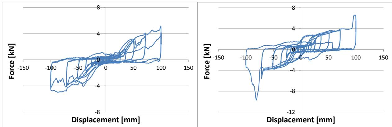
Fig. 8. Typical hysteretic response of hammer-head strap connections with: a) hot rolled channels, b) cold formed channels
