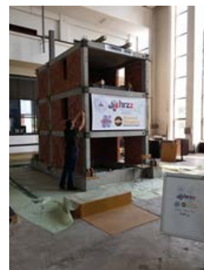
Fig. 1 – Tested composite framed-masonry structure (measures in cm)
