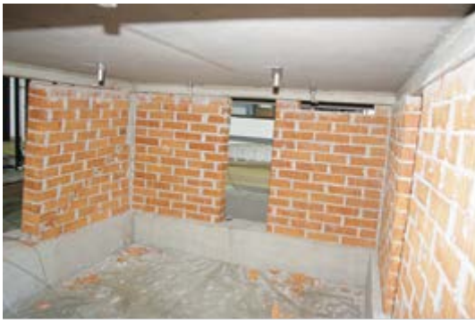
Fig. 4 – Damage of the framed-masonry wall with opening due to exposure to out-of-plane excitation
