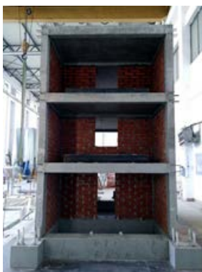
Fig. 1 – Tested composite framed-masonry structure (measures in cm)
