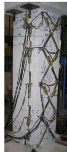
**Fig. 4-** Deformation measurement
