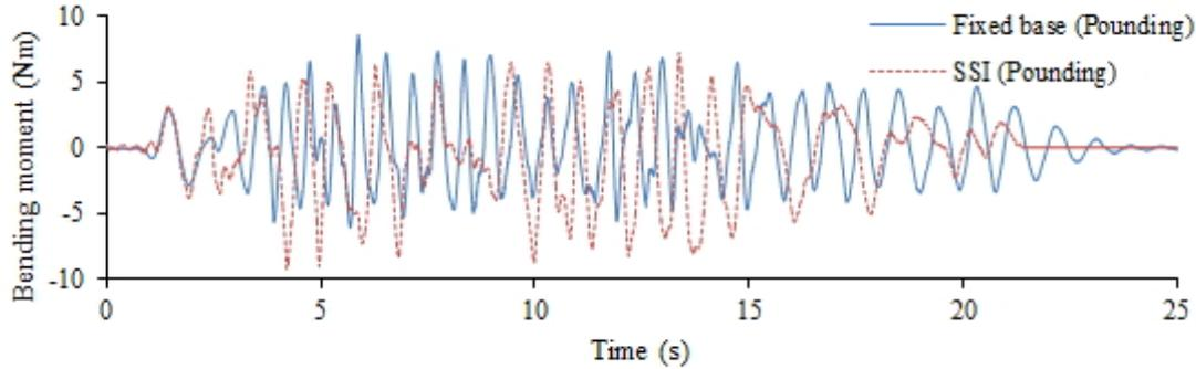
Fig. 6 – Bending moment of 30° skewed bridge for fixed base and SSI case considering pounding
