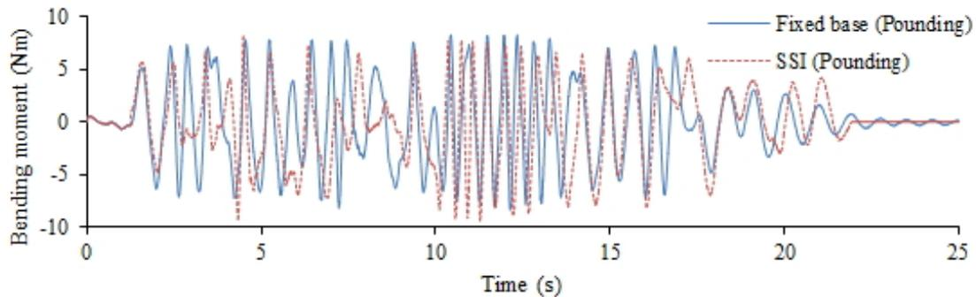
Fig. 4 – Bending moment of straight bridge for fixed base and SSI case when considering pounding
