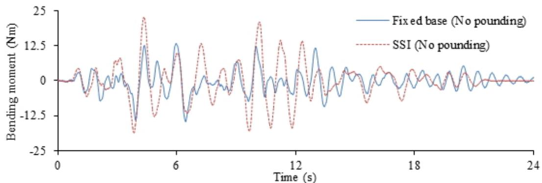
Fig. 5 – Bending moment of 30° skewed bridge for fixed base and SSI case without pounding
