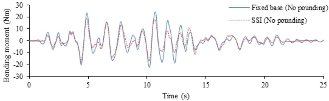
Fig. 3 – Bending moment of straight bridge for fixed base and SSI case without considering pounding
