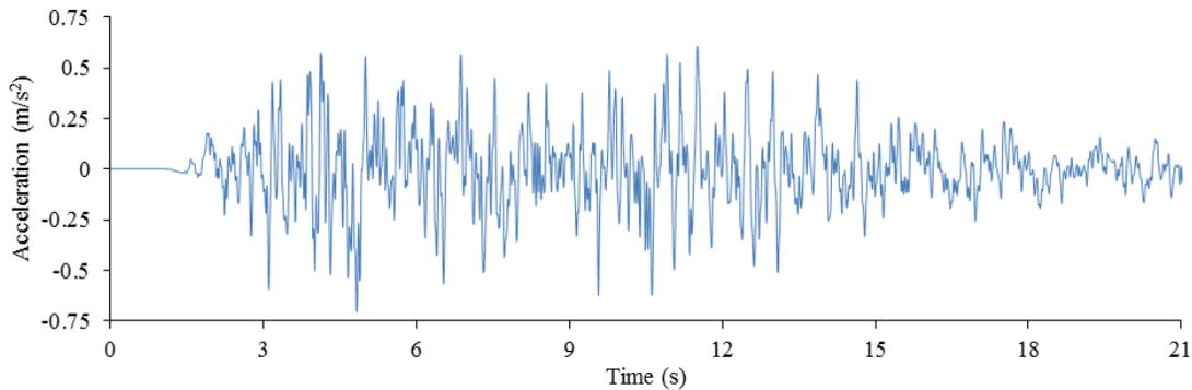
Fig. 1 – Acceleration time history of ground motion applied to model
