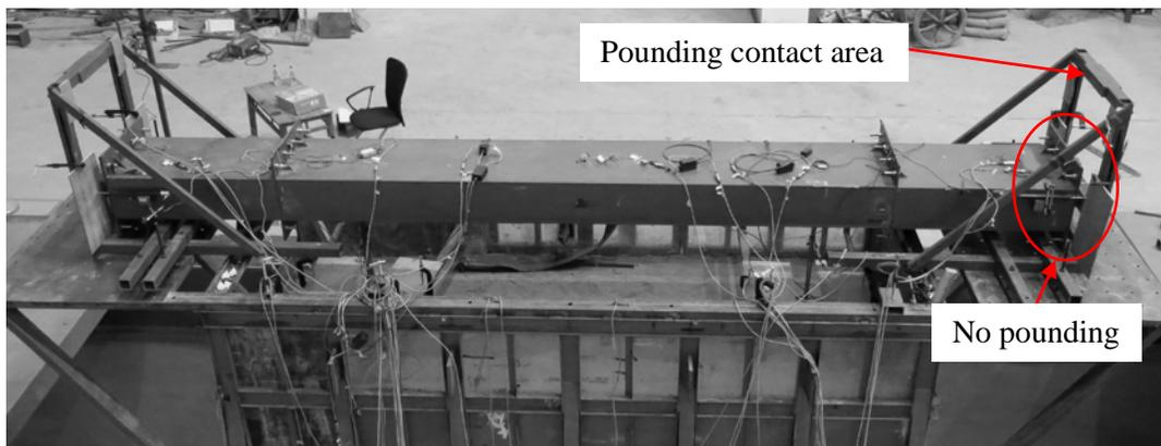
Fig. 2 – Setup of straight bridge for SSI case without considering pounding
