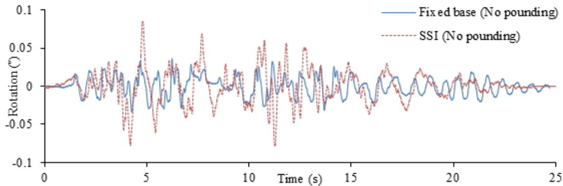
Fig. 7 – In-plane rotations of 30° skewed bridge for fixed base and SSI case without pounding
