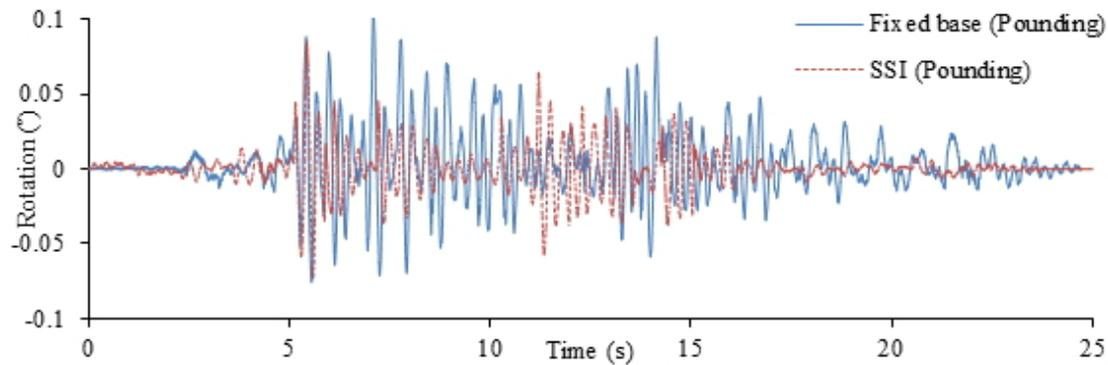
Fig. 8 – In-plane rotations of 30° skewed bridge for fixed base and SSI case with pounding
