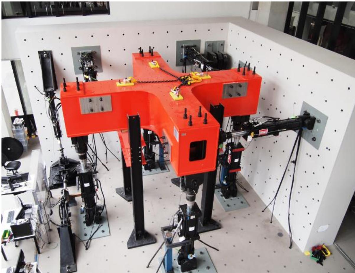
Fig. 1 – Multi-Axis Substructure Testing (MAST) system in the Smart Structures Laboratory at Swinburne University of Technology, Melbourne, Australia
