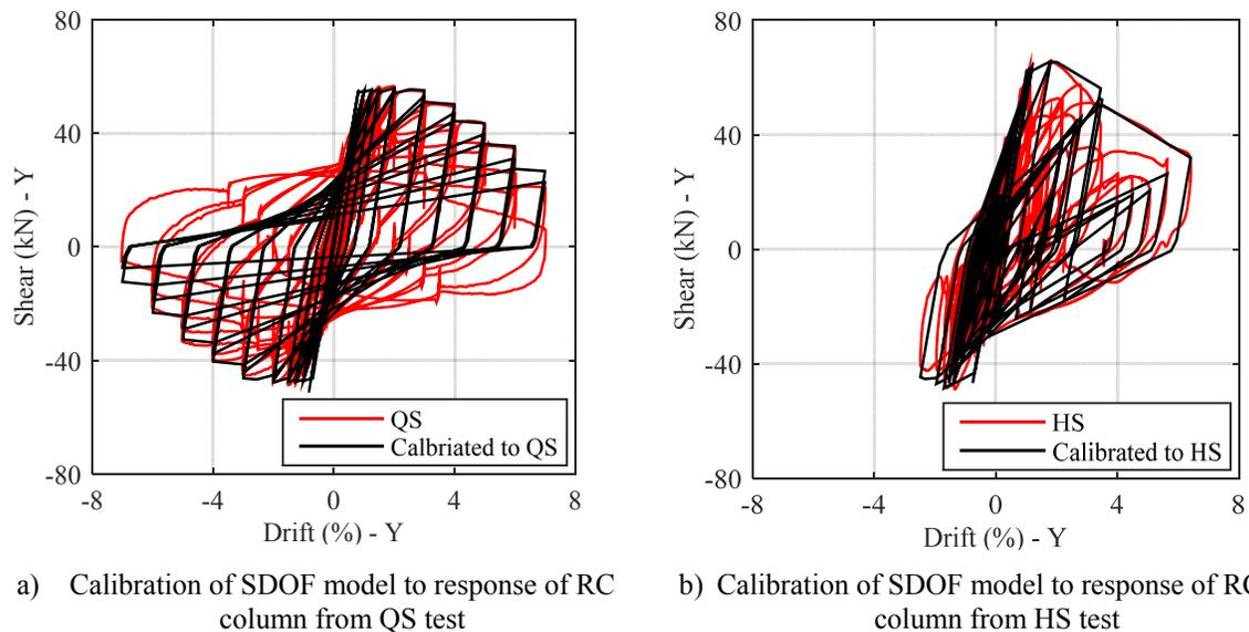
Fig. 6 – Calibration of SDOF numerical model to QS test results and comparison with HS test results
