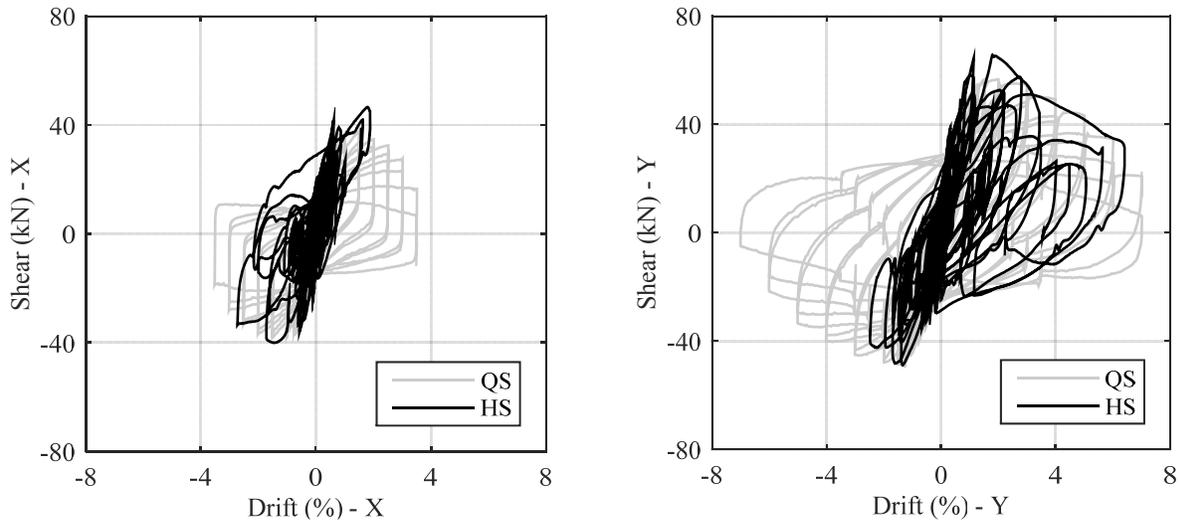
a) Comparison of the responses of RC columns in X and Y axes
