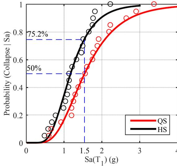
Fig. 8 – Comparison of fragility curves for the RC column based on results from QS and HS tests
