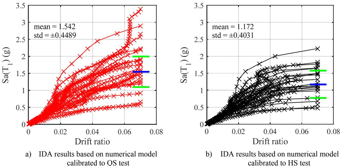
Fig. 7 – Comparison of IDA results for the RC column based on results from QS and HS tests
