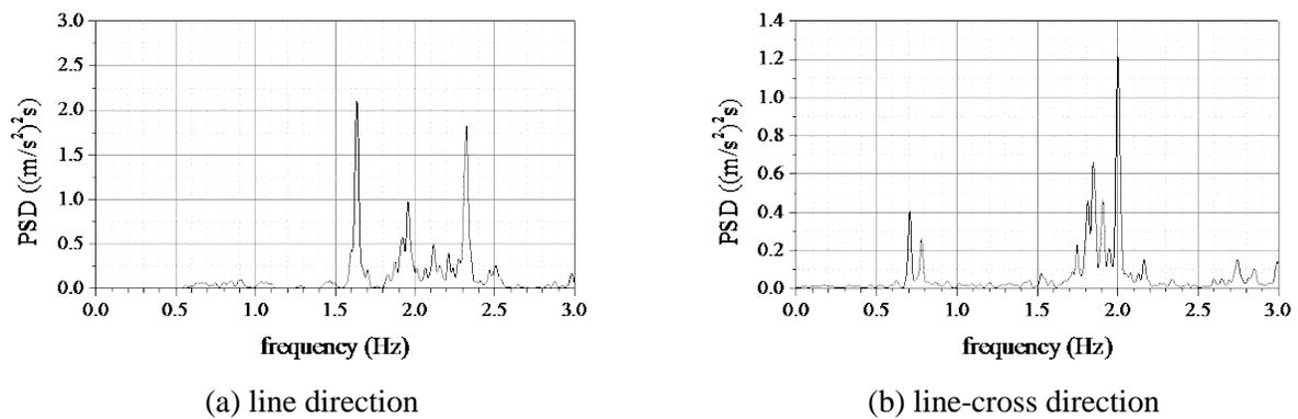
Fig. 6 – Power spectral density function of tower top acceleration
