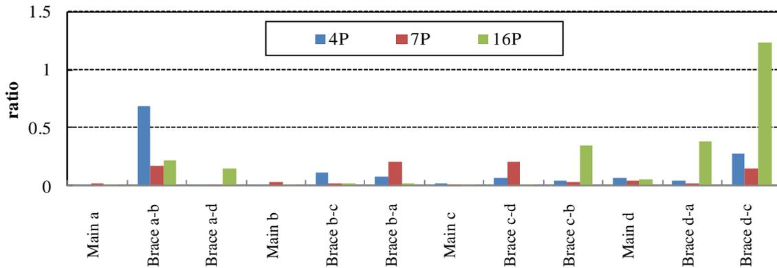
Fig. 13 – Gap of a center of axial force before and after earthquake
