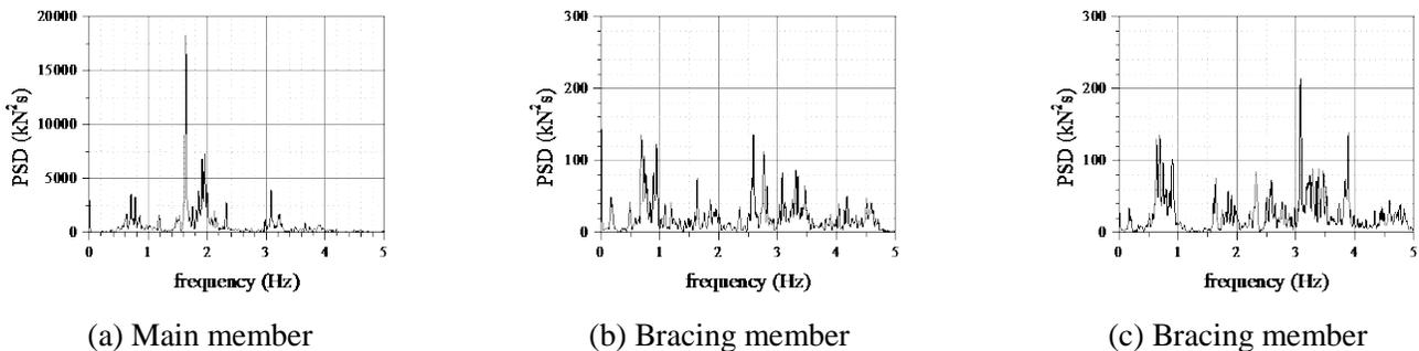
Fig. 10 – Power spectral density functions of tower member axial force
