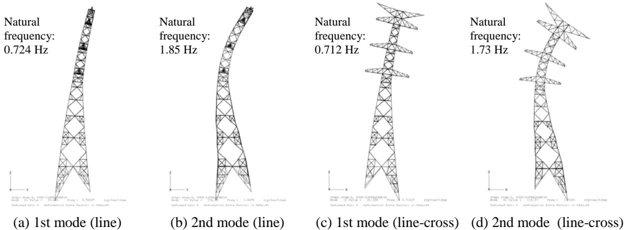
Fig. 9 – Mode shapes of target tower
