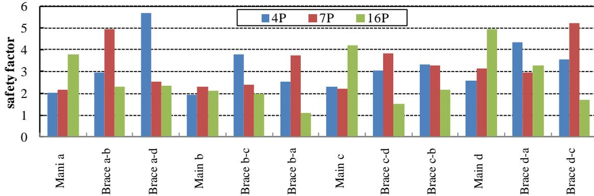
Fig. 11 – Safety factor of tower member during earthquake
