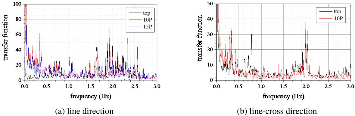
Fig. 7 – Transfer function between tower top response and ground motion
