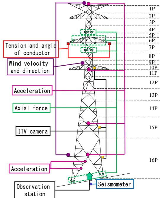
Fig. 2 – Measurement positions
