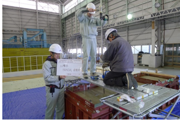
Photo 2 - Cone penetration test with a variable energy dynamic cone penetrometer in the container.
