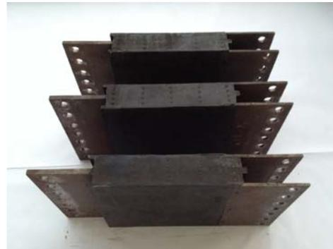
Fig.2 High-damping Rubber Damper
