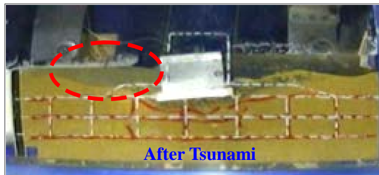
Fig. 7 Breakwater after tsunami overflow
