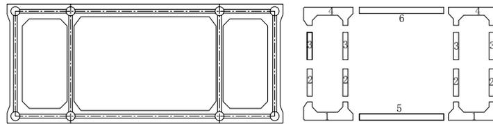
Fig.5 Section and construction sequence number of the arch rib
