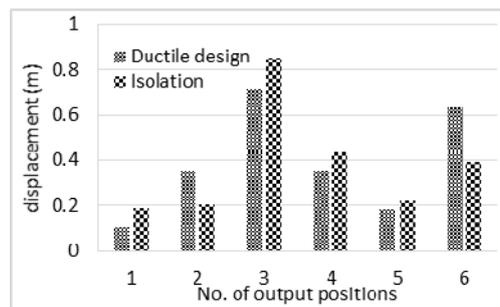
Fig. 11 Lateral displacement demand of girder under rare earthquake (Unit: m)
