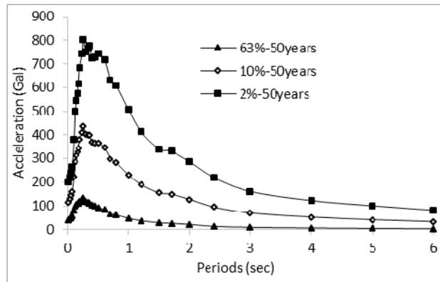
Fig.1 Response spectra accelerations with a 5% damping ratio
