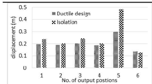
Fig. 10 Longitudinal displacement demand of girder under rare earthquake (Unit: m)
