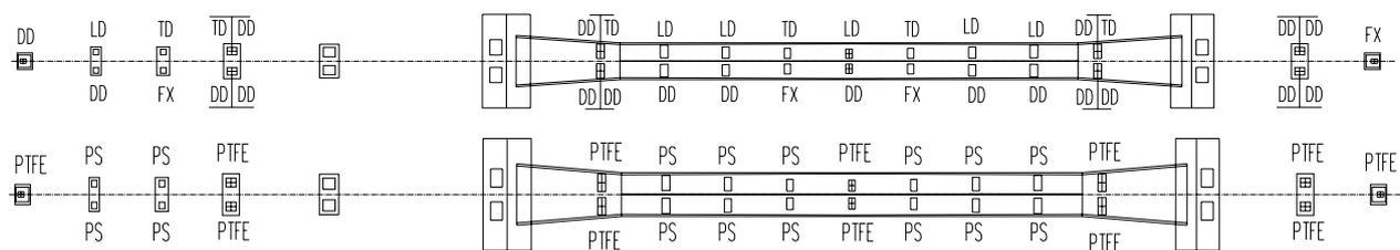
Where, DD denotes double-direction movable, LD longitudinal direction movable, TD transverse direction movable, FX fixed bearing, PTFE denotes Teflon sliding bearing movable, PS denotes spherical steel bearing.
