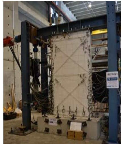
(a) Test setup illustration (b) Photo of test setup in lab Fig. 3 - Test setup used to achieve the desired test moment to shear ratio
