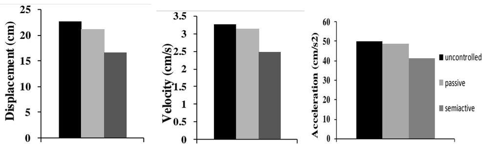
Fig. 3 – Peak displacement, velocity and acceleration of the top storey for uncontrolled, passive controlled and the semi active controlled cases
