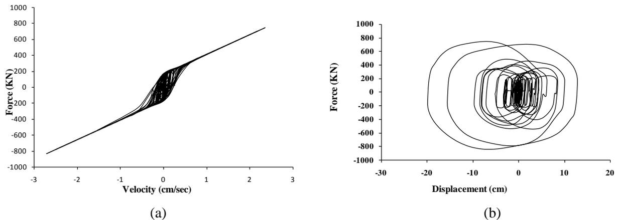
Fig. 5 – Controlled responses for the fifth storey MR damper : (a) force versus velocity and (b) force versus displacement.
