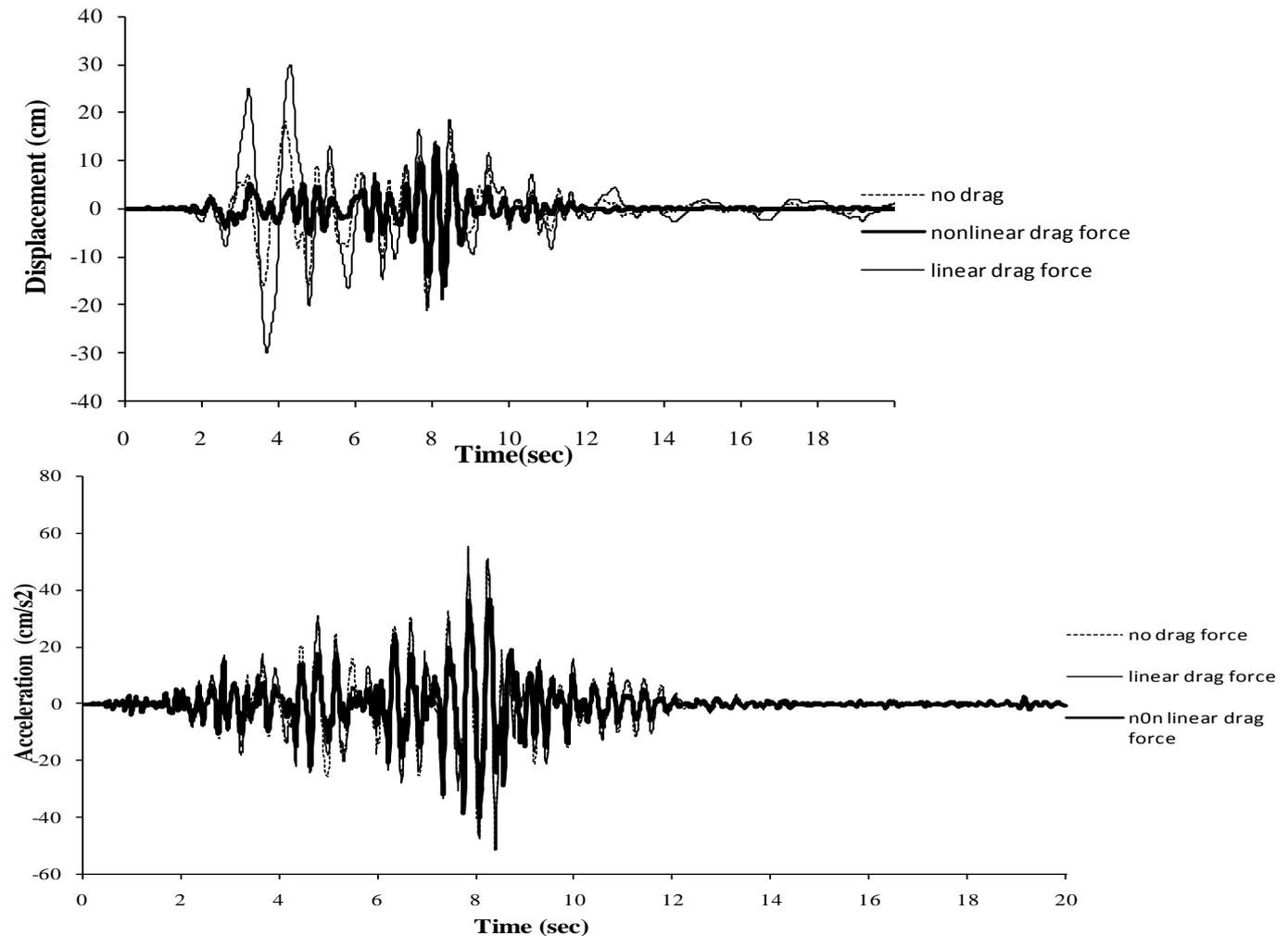
Fig. 9 – Effect of drag force on the control of fifth floor responses: (a) displacement and (b) acceleration.
