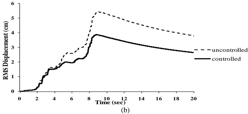
Fig. 4 – Top floor responses of the jacket platform under San Fernando earthquake excitation: (a) absolute acceleration and (b) RMS displacement
