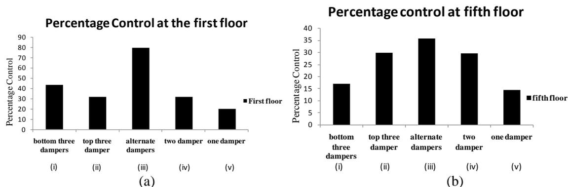
Fig. 2 –Percentage control of displacements at (a) fifth floor and (b) first floor of the offshore jacket structure subjected to San Fernando earthquake ground motion.
