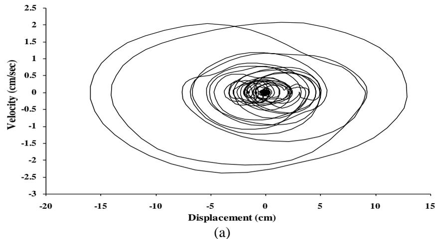
Fig. 7 – Phase plane plots (controlled displacement versus velocity) of fifth floor
