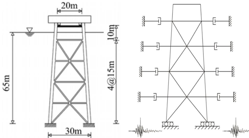
Fig. 1(a) – Steel jacket platform & (b) – Water structure interaction of the steel jacket platform
