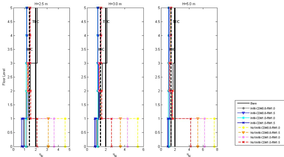
Fig. 6 – Nonlinear Pushover Analysis Results for Frames with Different First Story Heights and with Table 3 variables.
