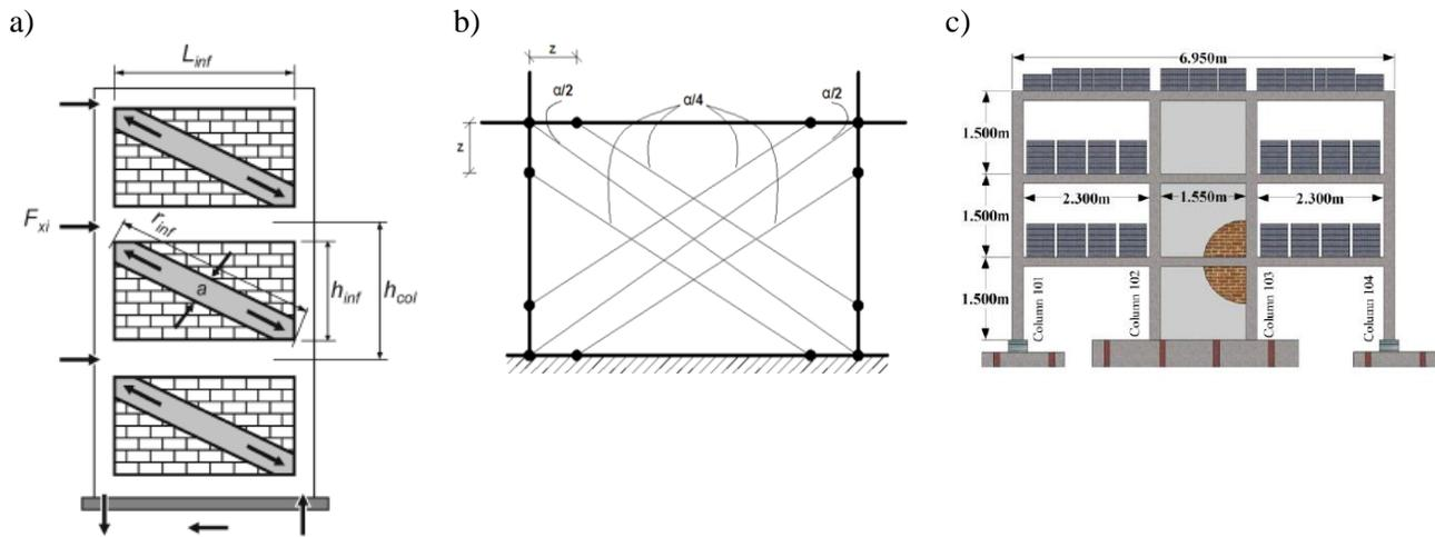
Fig. 1 – a) ASCE41 Concentric compression strut model b) three strut model c) METU Specimen (Fenerci 2013)
