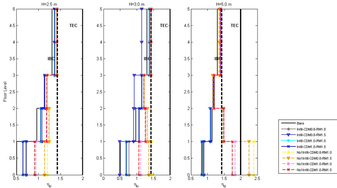
Fig. 5 – Mod Superposition Analysis Results for Frames with Different First Story Heights and with Table 3 variables.
