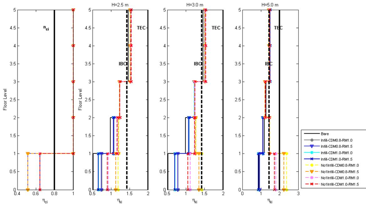
Fig. 4 – Linear Procedure Results for Frames with Different First Story Heights and with Table 3 variables.
