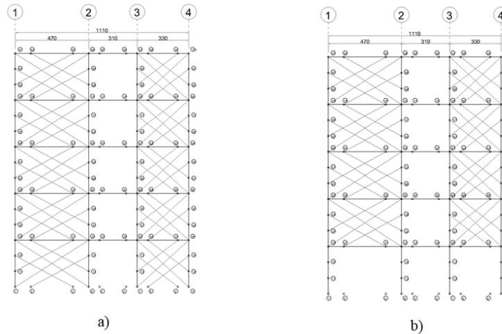
Fig. 3 –a) Infills at each story (“Infill” in Figures), b) Infills at each story except first story (“No1Infill” in Figures)
