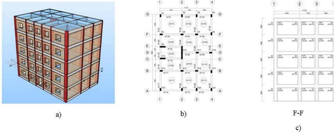
Fig. 2 – 5-story, a) 3D view, b) plan, c) FF axes frame
