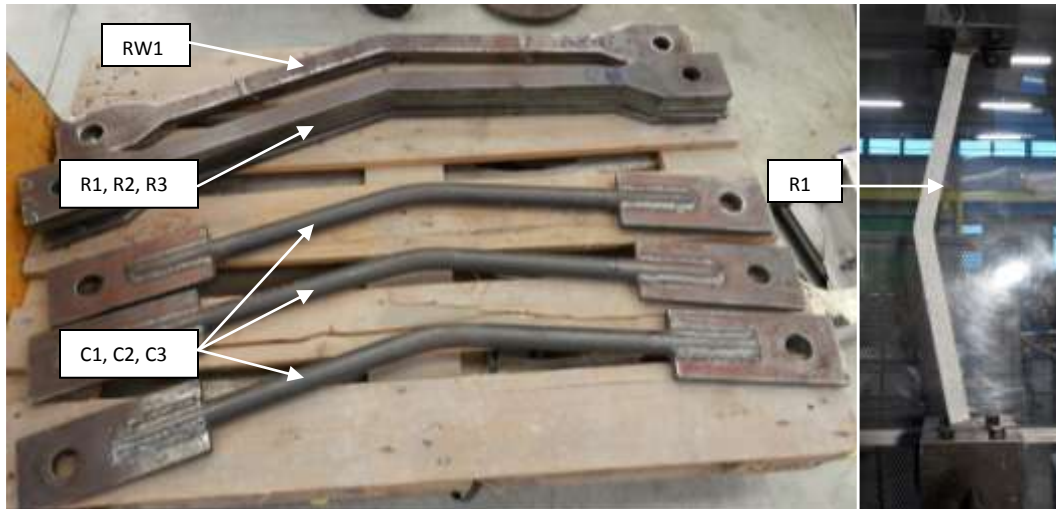
Fig. 3 – The CSB specimens: left) before the test, right) under test
