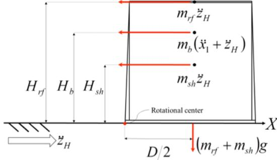
Fig. 4 – Forces at the initiation of the tank rocking motion
