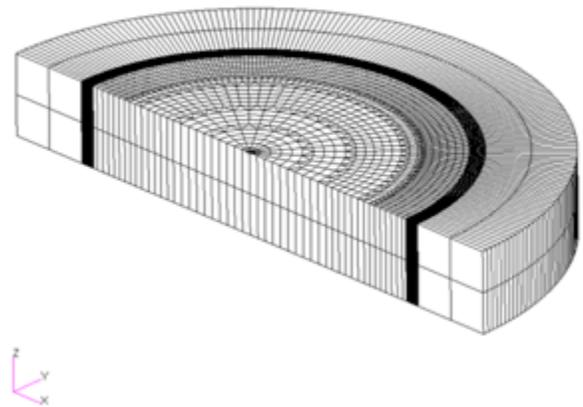
Fig. 6d – Numerical model of foundation
