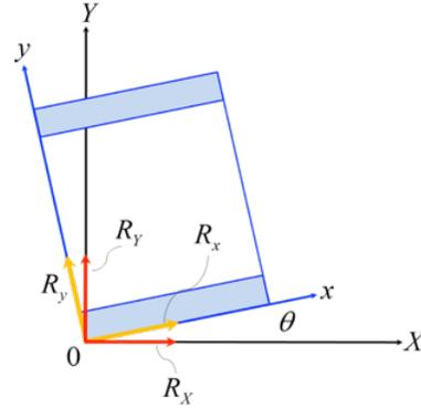
Fig. 1 – 2DOF model in displaced and rotated position
