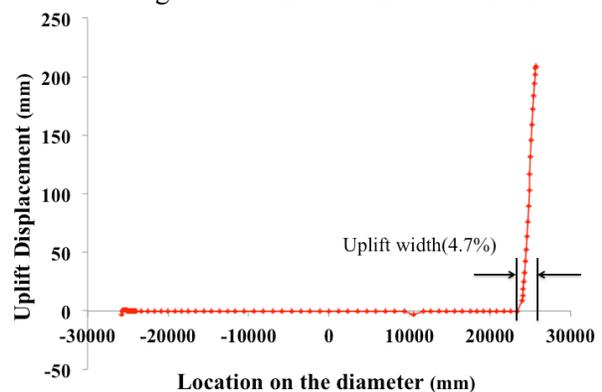
Fig. 7b – Uplift width of the tank bottom plate (t = 2.3s)
