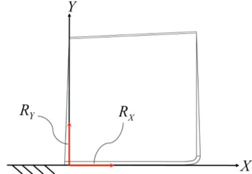
Fig. 5 – Base shear and reaction during the tank rocking motion
