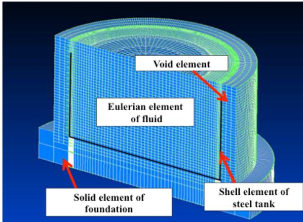
Fig. 6a – Numerical tank modeled in LS-DYNA
