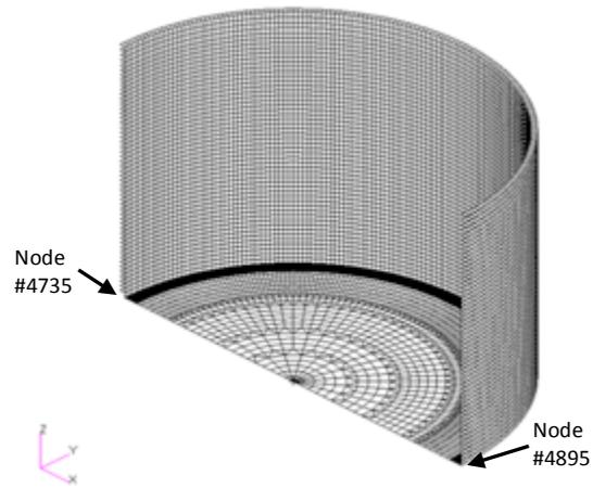
Fig. 6b – Numerical model of shell and bottom plate
