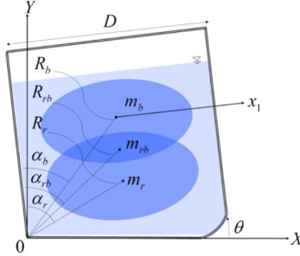
Fig. 3 – Analytical model of tank rocking motion
