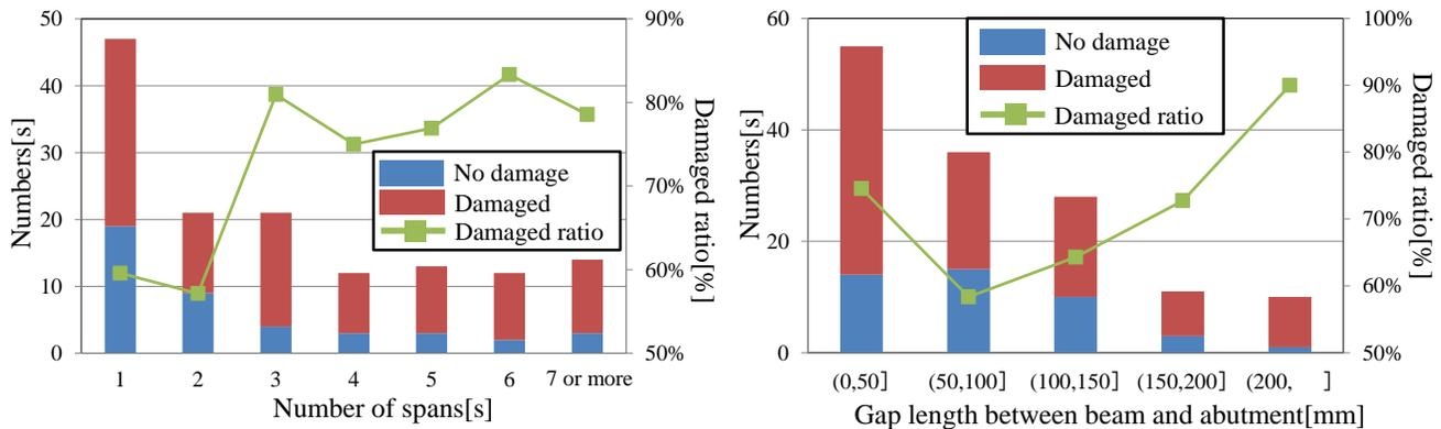
Fig. 6– Damage case analysis by the result of on-site investigation
