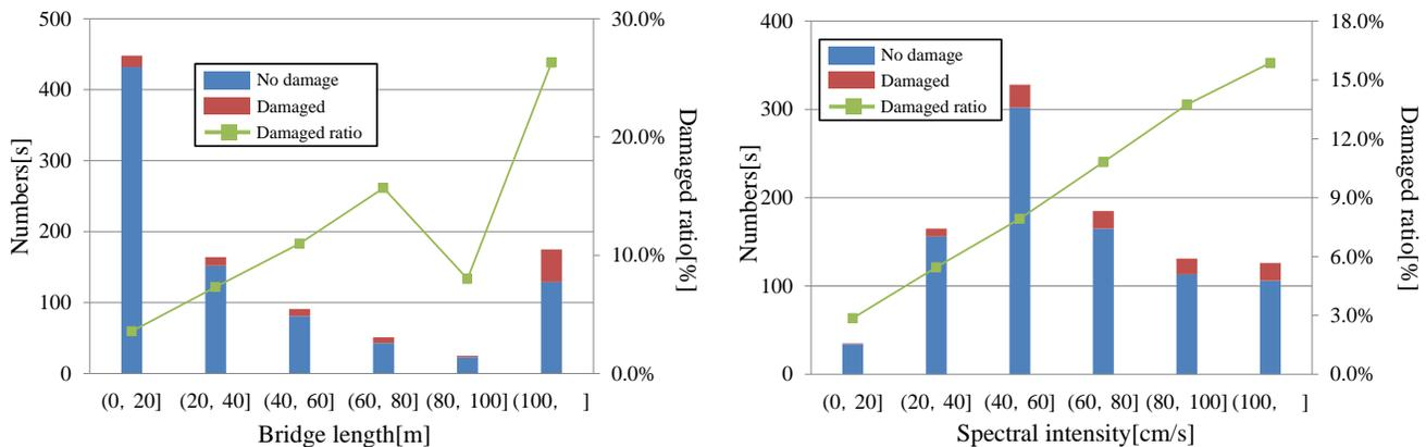
Fig. 4– The damage analysis by bridge length and spectral intensity
