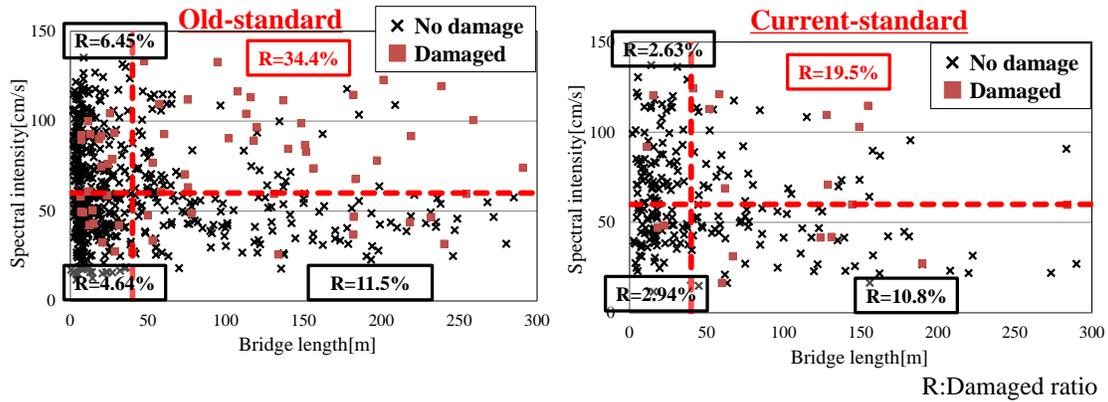
Fig. 5– The damage analysis by bridge length, spectral intensity and kind of joints
