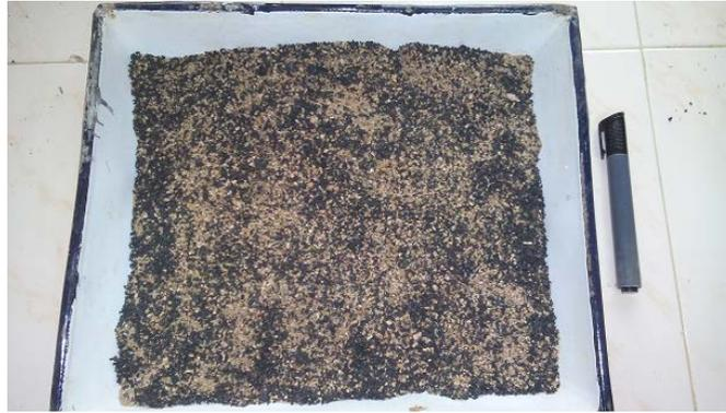
Fig. 2 – Soil-tyre mixture used for the cyclic triaxial test
