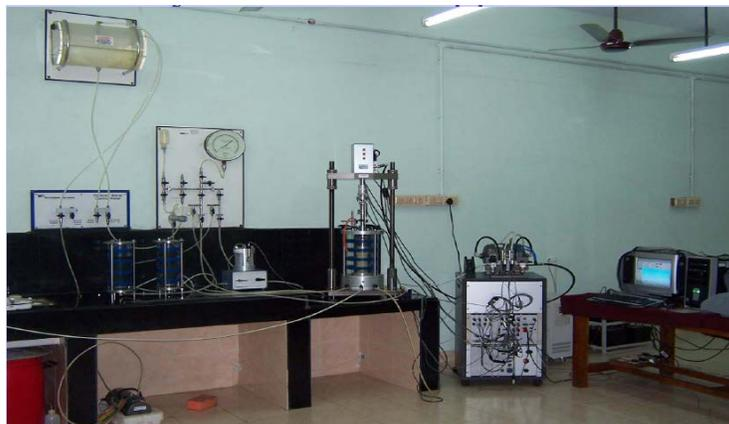
Fig. 3 – Cyclic triaxial test setup
