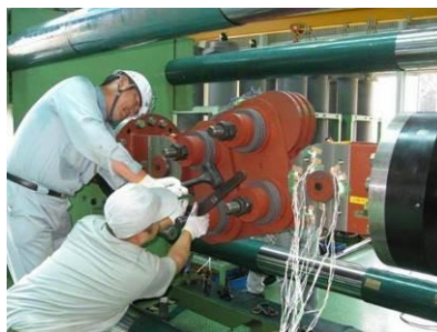
Figure 17 - Test setup of 1500 kN damper in testing facilities in Japan
