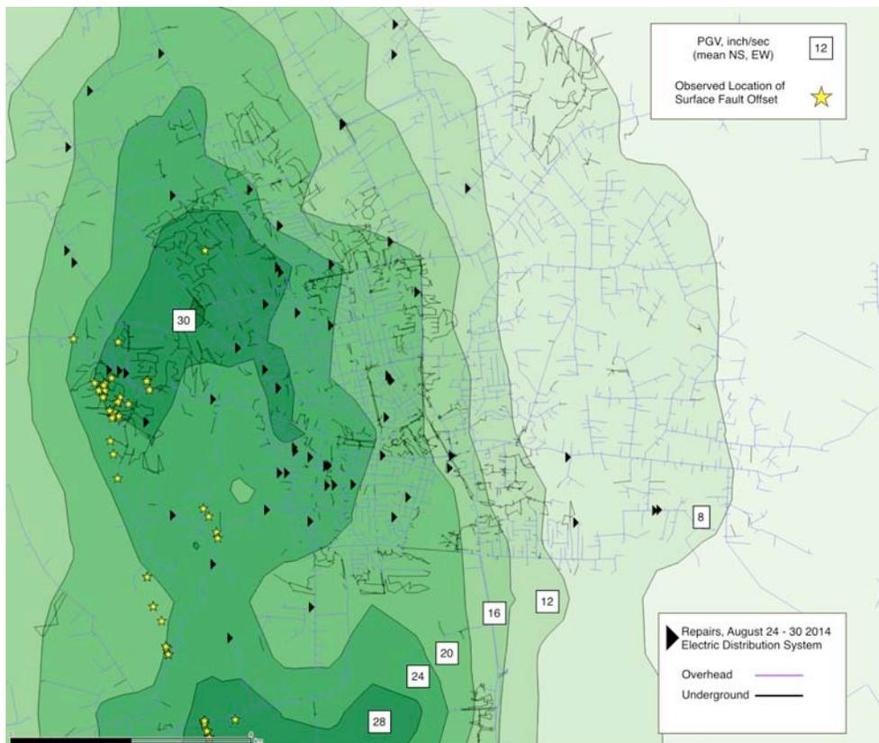
Fig. 5 - Electric Distribution System Repairs near the City of Napa
