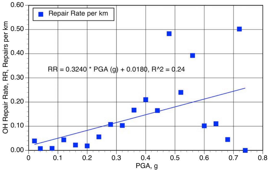
Fig. 6 - Repair Rate, Overheads, Using PGA
